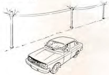
AM - SUSCEPTIBLE TO POWER LINE NOISE
