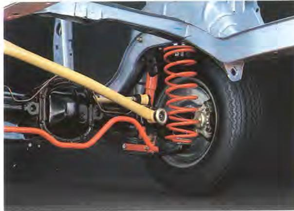
tion and braking, and a "panhard" rod which holds the axle laterally. Coil springs, a stabiliser and shock absorbers complete the picture.
