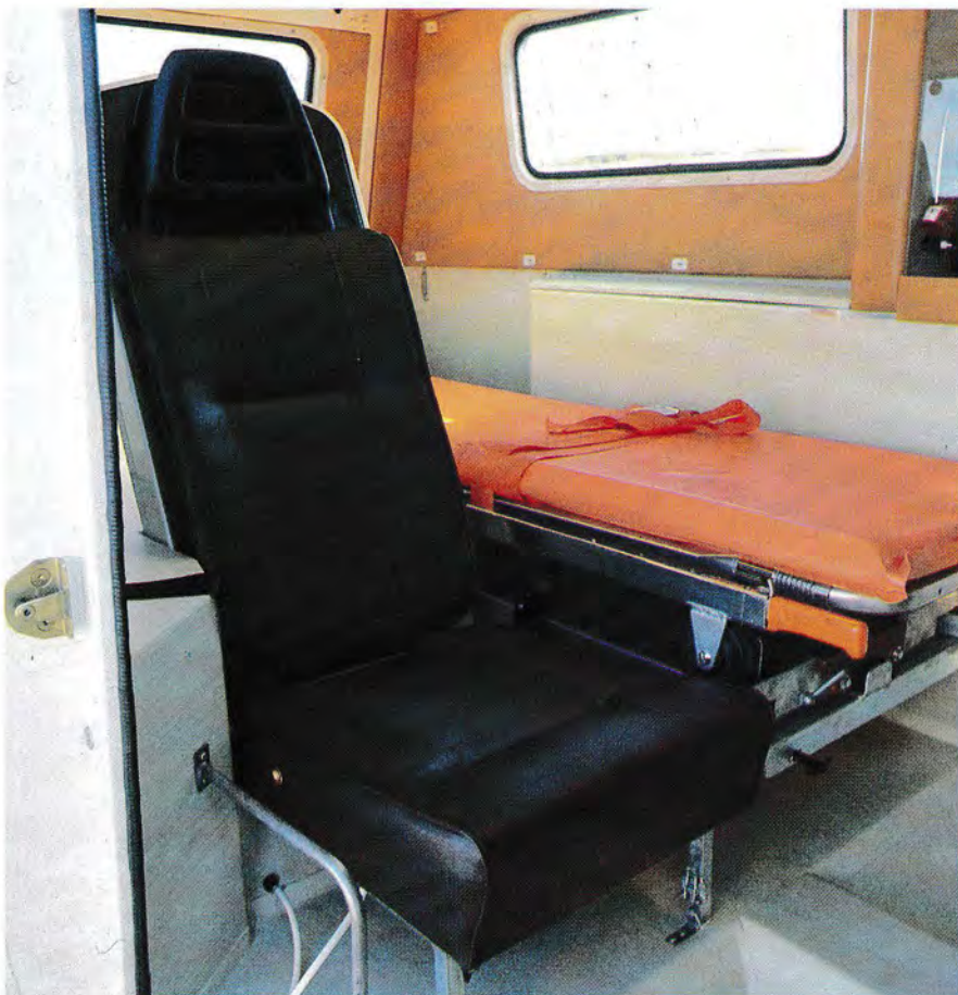
The functional and comfortable attendant's seat comes with a high back as well as a built-in head restraint for extra safety. The seat, which folds down, also comes fitted with an inertia reel seat belt.
