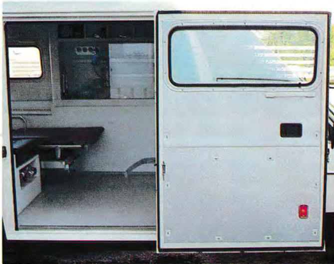
The wide side door facilitates entry and exit for the personnel. It can also be used as an emergency exit in the event of the ambulance being run into from behind.
