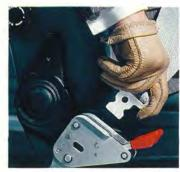
If you want people to use something, make it easy. We made Volvo seat belts very easy to use. Once adjusted they snap solidly in place without further adjustment. Three-point belts are standard equipment up front. In the back, three-point anchorages are already installed for the two outside passengers, with lap belt anchorages for the middle passenger.
