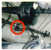
The steering column is designed to break away under severe impact. This eliminates danger of the steering column being forced back toward the driver in case of head-on collision.
