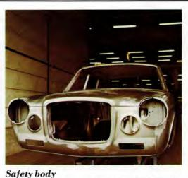
All-welded integral construction steel body made up of large all-pressed sections. Assembled by means of about ten thousand spot welds. (Every spot-weld is powerful enough to carry the entire weight of the body.) Energy-absorbing front and rear ends. Around every opening in the body there are reinforcing members with closed profiles. The roof is also reinforced by means of cross-members.
