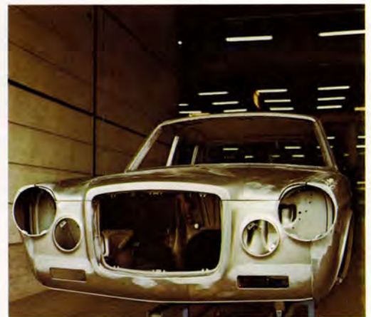
Safety body The Volvo 164 is designed with energy-absorbing front and rear ends. We don't only claim this: we tested it before we began producing the 164. We drove a prototype into a wall at 30 mph. The front end was crumpled but the passenger compartment remained completely intact.
