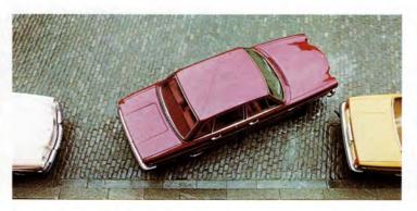
The turning circle diameter is 9.6 m (31'6"). When using full wheel lock, for instance when parking, the steering gear ratio alters and takes the weight of your arms.
