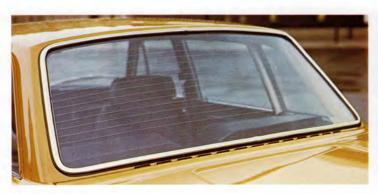
The rear window has fine heating wires embedded in the glass. The selector switch has two positions, 75 W or 150 W to meet all requirements. Below the window are air extractor vents which provide draught-free ventilation and better heating or cooling, as the case may be.
