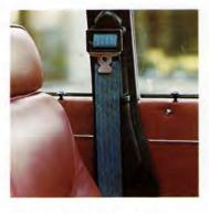
Up front the Volvo 164 has factory-fitted three-point safety belts of inertia type. The seat belt furling reel is ideally located and recessed in the door pillars. Unobtrusive. Nothing to trip over. Snap-action locking tongues.
