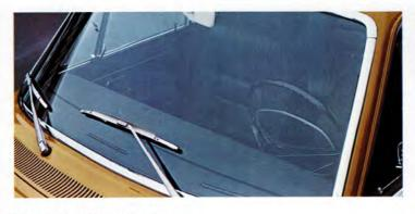
The windscreen is of highimpact type and features a tough intermediary safety layer of plastic. This is the very best available. A windscreen of this type is shock-absorbing and ensures clear vision even when hit by flying stones. The windscreen wiper on the driver's side is of an aerodynamic anti-lift type which keeps the blade firmly pressed against the glass even at high speeds.
