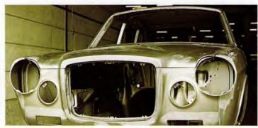
A safe body. Integral, all-welded steel. Composed of large one-piece sections fused together by approximately ten thousand spot welds. Energy absorbing front and rear ends. Reinforced box-section safety profiles round all body openings. And to top it all, even the roof is reinforced with traverse roll bars. All doors feature burst-proof locks.
