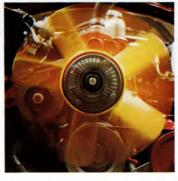
The engine cooling fan is driven through a viscous slip-type coupling which limits fan speed to max. 3,500 r.p.m. This reduces both engine noise and fuel consumption as well as increasing net output and reducing warming-up times.
