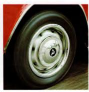
Big wheels make short work of bad roads. The Volvo 164 has 165SR15 radial tyres. These tyres are meant for high-speed work.
