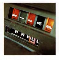
Of course, you can also specify an automatic transmission. This is a fully-automatic unit with part throttle change-down to give you immediate response in city traffic and faster cornering.
