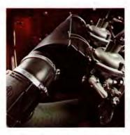
Fuel is supplied through twin horizontal carburetors adjusted and sealed at the factory for Volvo's "dual-induction" emission control. Induction air is thermostatically controlled to a constant temperature by a preheating system in line with the air cleaner.
