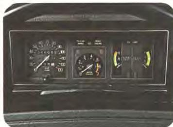
Dashboard instrumentation is clock-like and easily read. The tachometer is for those who want to know the speed of their engine in addition to the speed of their car.
