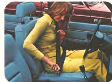
Self-adjusting three-point lap/shoulder seat belts are standard. They flex enough to permit normal movement but tighten up in a sudden stop.
