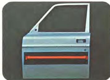
A steel tube is welded into every door to protect against sideswipes. Elimination of the vent windows has quietened the interior and strengthened the front doors.
