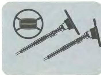
In case of front-end impact, a section of collapsible steering column telescopes on itself. Pressure against the steering wheel moves it into a vertical position against which the driver's weight is more evenly distributed.
