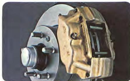
There's a power-assisted disc brake for each wheel. Discs resist "fade" due to heat build-up better than drum brakes. Front discs are specially ventilated to dissipate heat that can exceed 1100° F.
