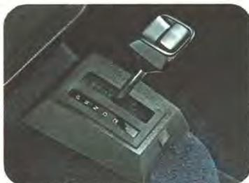
A trigger on top of the selector lever for the three-speed automatic transmission is designed to prevent you from shifting into "R" from "D" at 60 mph. And engaging a substantial repair bill.
