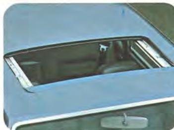
The steel sunroof (our only factory-installed optional extra) cranks open to let in more than three-square-feet of sunlight. And closes flush with the roof.
