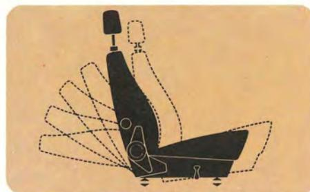
The bucket seat has a 7<sup>3</sup>/<sub>4</sub>" travel front-to-rear while the backrest reclines from vertical to nearly flat out. New locking devices make these adjustments permanent. Until a new passenger wants to re-adjust them.
