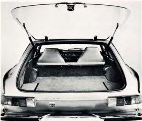
For easy access to the rear compartment the rear window of the 1800 ES can be fully opened.
