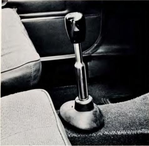
New remote control gearshift lever for more positive gear selection.
