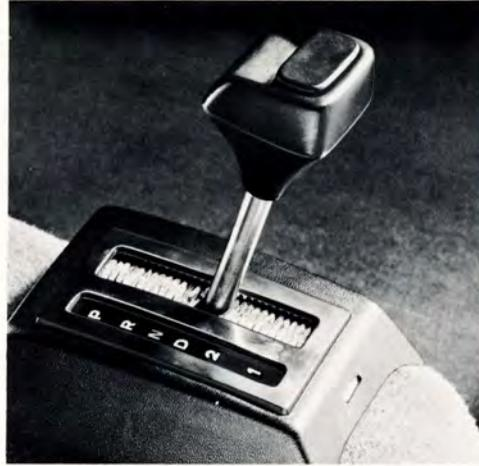
Automatic transmission equipped with a floor mounted gearshift lever with push button selector lock in the gear lever knob. New 6 position pattern: PRND21 and re-designed transmission which allows driver to have manual control or the convenience of full automatic.
