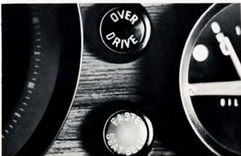
An additional safety feature on the Volvo 1800 E/ES is a warning light on the dashboard which reminds the driver to fasten his safety belt.
