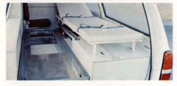
The folding extra stretcher is stored in an easily accessible location. The right-hand seat for personnel folds down and provides a support for the two telescopic rails on the extra stretcher which can easily be slid out.
