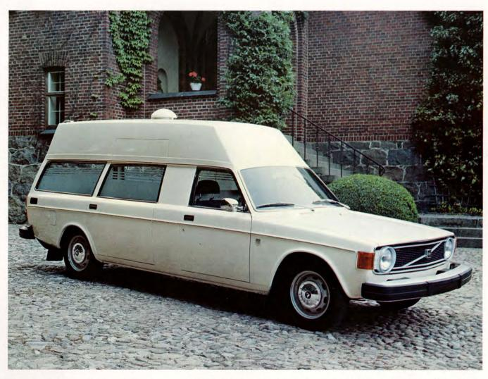
The completely new Volvo ambulance is based on the same design as the Volvo 145. The height and length of the body, however, have been considerably increased in order to provide a spacious and functional interior. The right-hand rear door extends into the raised roof in order to facilitate rapid entry and exit for ambulance personnel. The entire patient accommoda-
