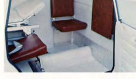
The seat for ambulance personnel to the right of the main stretcher is fitted with a safety belt and can be adjusted to two positions. In the forward part of the ambulance accomodation there are also two folding seats.
