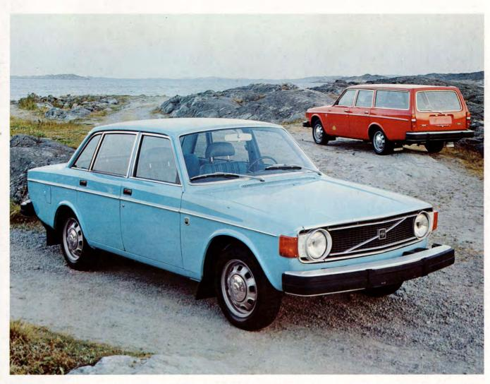
Most of the models in the Volvo 140 Series can be provided in a special version for those suffering from physical handicaps. Versions with A-engines can now be obtained with a completely new pneumatic power assembly for throttle and brake operation. The exterior and basic design are the same as on the standard cars. The models this year are characterized externally by the new deep bumpers
