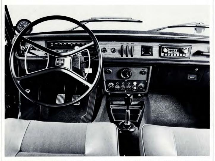
The comprehensive instrumentation includes the following extras: switches for siren, rotating roof lights, engine compartment and luggage compartment lighting and reversing light. There is also a control for the automatic lighting switch: the parking lights go on automa-
