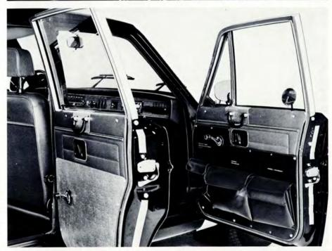
The rear doors are fitted with aluminium kick plates. Front door pockets hold leg and arm reflectors, stop signs, traffic control cuffs, document file, tyre pressure gauge, tools. All doors are fitted with folding handles, the rear doors also having catches which can be locked from the front seats.
