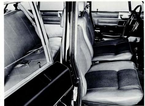
The front seats have firmer stuffing in the cushions and backrest. Reinforced and particularly durable upholstery. On the rear of each backrest there is a pocket for night duty coats. Tubular retainers under seats for batons.
