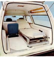
The basic design is that of the Volvo 145 Express with a 90 b.h.p. SAE engine and a 4-speed manual gearbox. Safety features are the triangle-split dual circuit brake system, the collapsible steering column and the adjustable head restraints — all examples of Volvos endeavour to increase, road safety. The excellent running economy, good performance and functional comfort give a car which can stand any amount of rough treatment.
