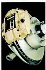
furnishes 30% of the car's total braking power while each rear wheel supplies 20%, you always have 80% of the car's braking power working for you even if one system fails.
