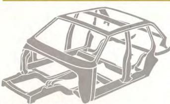
Each of the six steel pillars holding up the roof is strong enough to support the weight of an entire car. Turn that over in your mind.
