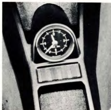
Oddments console with electric clock on propeller shaft tunnel.
