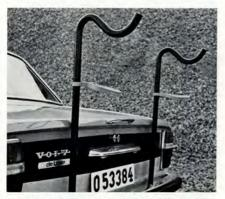
Volvo Taxis can also be specified with a cycle carrier. The carrier has a plastic veneer and is also designed to carry mopeds. Two holding straps are also included.
