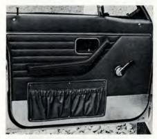
The inner door panels are also clad with vinyl and the lower section is protected by a kickplate. Extended kickrails of aluminium protect the door sills. Door opening angle is no less than 80°.
