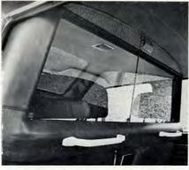
The front and rear areas are divided by a sliding screen of laminated glass. Fitted with a securing catch of course. The dividing screen framework is safety padded and clad with hard-wearing vinyl. The Volvo Taxis can also be supplied without this dividing screen. The front seats have head restraints.
