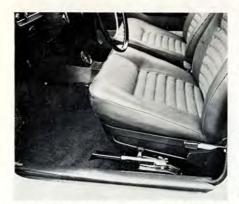
The driving seat has a very wide range of adjustability. The seat stuffing is extraresilient and the seat webbing is of heavyduty type. The seat cushion is upholstered in cloth and the side panels are of vinyl material. The well grouped instrumentation and controls are easily identified and used.
