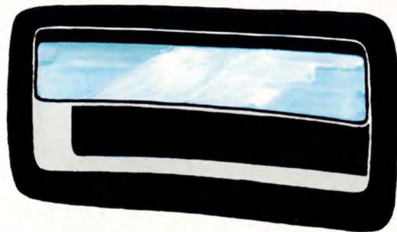
The door handles are recessed. This is not just styling – it is also a safety detail. Another safety detail is that the rear doors of our four-door saloons can be locked so that they cannot be opened from the inside – which means you can have an easy mind with children in the car.
