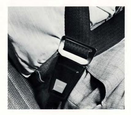
Buckled belt on a rear seat passenger shows how the automatic adjustment feature assures proper fit.
