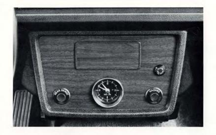
The safety system includes a dashboard warning light and buzzer, activated whenever the ignition is on and a gear is engaged, and/or the front passenger seat is occupied. The light and buzzer can only be shut off by fastening the safety belts.
