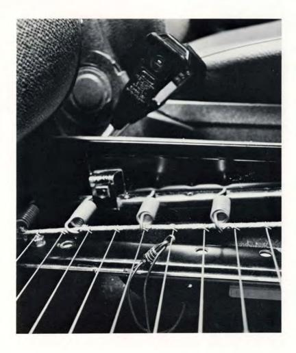
Sensor for the passenger seat is attached to a support strap under the cushion. It will activate the light and buzzer when weight is placed on the seat.
