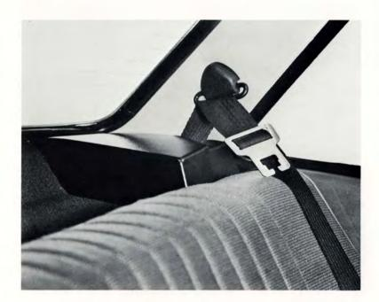
140 Series and 164 models have a new 3-point rear seat belt retracting mechanism on the rear shelf. This installation effectively eliminates the disorderly arrangement found in most cars and makes the belts even more convenient to use than a lap belt.
