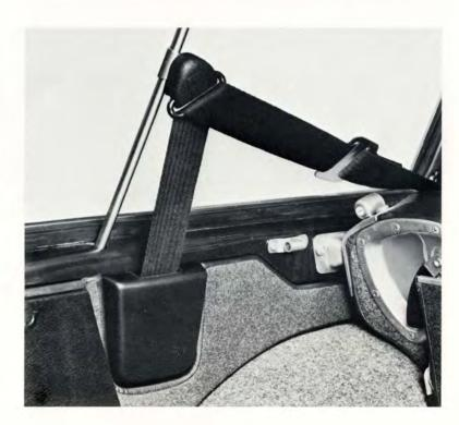
The rear seat retracting mechanism on the 145 is cleverly mounted to be out of the way and makes the belts easy to use. No longer will these belts be lost under the seat cushion. The vertical support bar positions the belt at the correct height.
