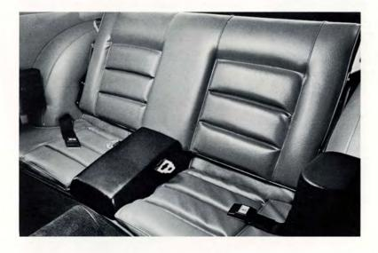
The rear seat of the 1800E/ES models has new retracting lap belts. The belts pull out from the retracting mechanism between the seats, a much improved convenience.
