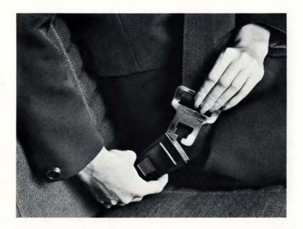
The rear seat 3-point belts fasten into a lock with a quick-acting release. There is a short length of webbing attached to the lock, and when not in use, the locking part lies on the seat cushion. There's a conventional retracting lap belt provided for a center rear seat passenger.
