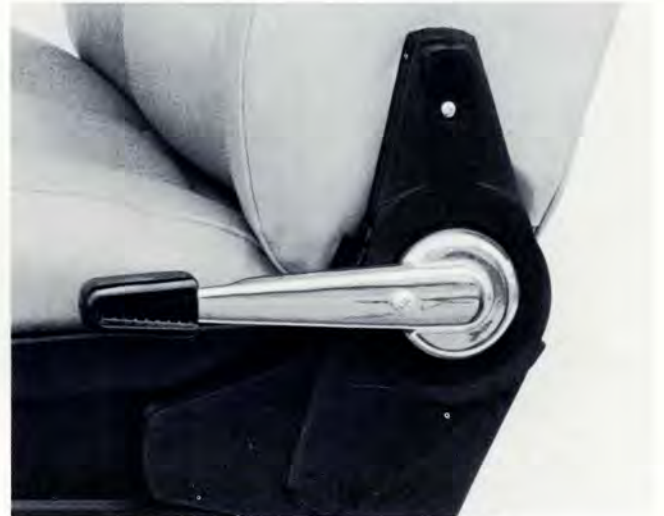
Lever on the outboard side of the seats adjusts the backrest to any position. This mechanism is part of an anti-whiplash device that will fold the seat back at a controlled rate if the 164 is struck from the rear.
