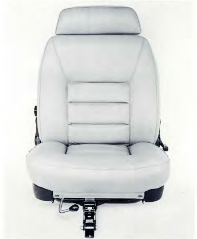
Lever on the outboard side of the seats adjusts the backrest to any position. This mechanism is part of an anti-whiplash device that will fold the seat back at a controlled rate if the 164 is struck from the rear.
