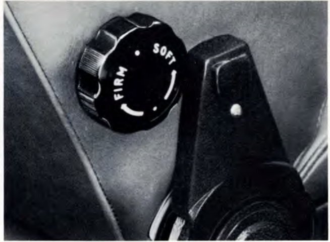
A knob on the side of the front backrest controls the tension of a wide horizontal strip inside the seat back. Volvo's exclusive lumbar support device provides comfort for a critical area, the lower part of an occupant's back.
