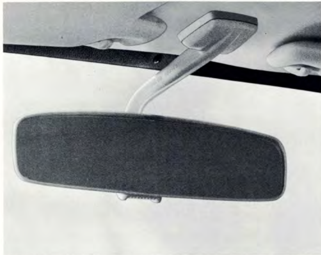
All Volvo models for 1970 have a breakaway, tinted interior mirror with an anti-glare feature operated by a slide on the bottom.
