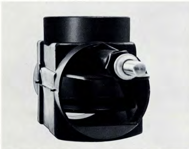
Flap valve in the coupling is positioned here with the forward branch closed, permitting only heated air to enter the carburetors.
