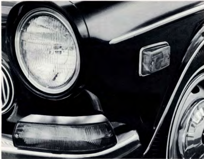
New for 1970 are illuminated side markers, amber in the front, red in the rear. Wraparound turn signals also are visible from the sides.
