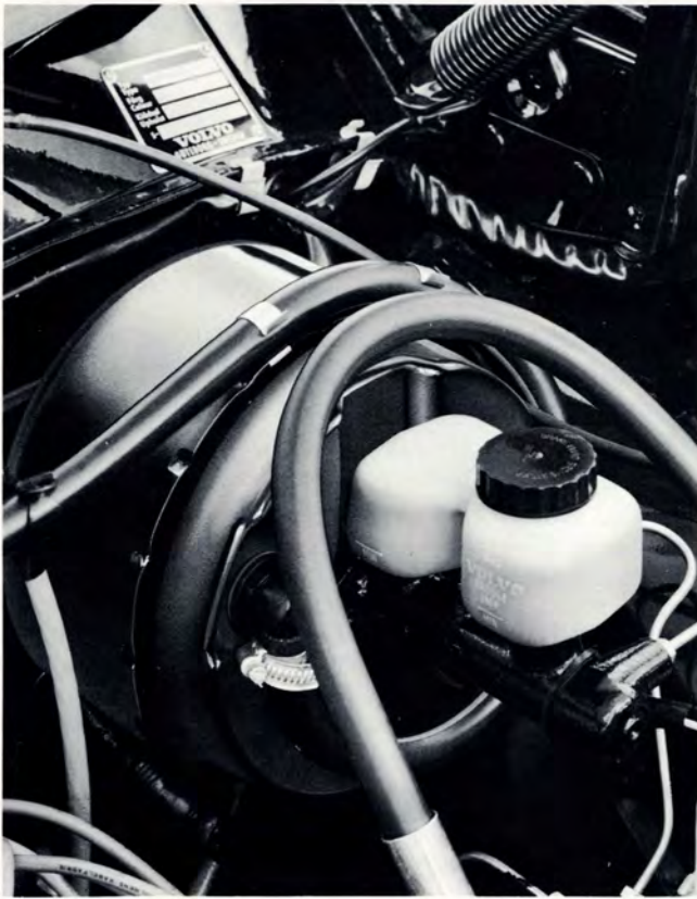
Power assist is standard on all Volvos. The 164 booster for the disc brakes has a powerful 1:4 reduction ratio.
