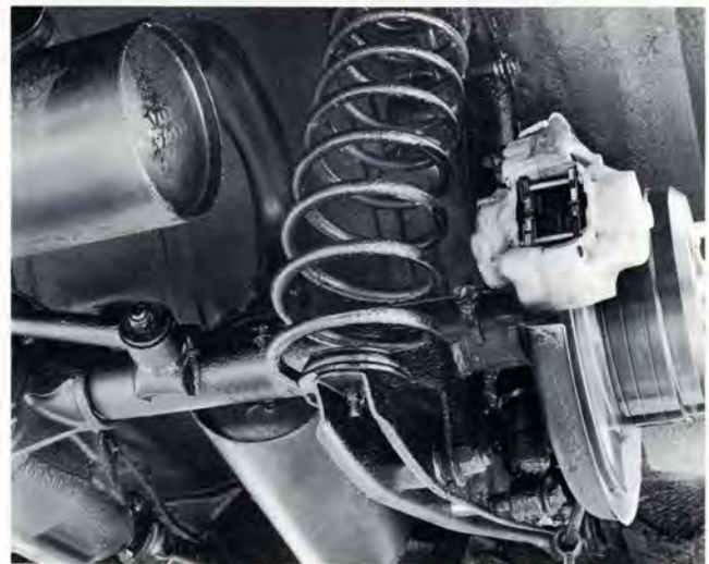
Volvo rear axles are carried by longitudinal control arms and torque rods to prevent axle shift.
