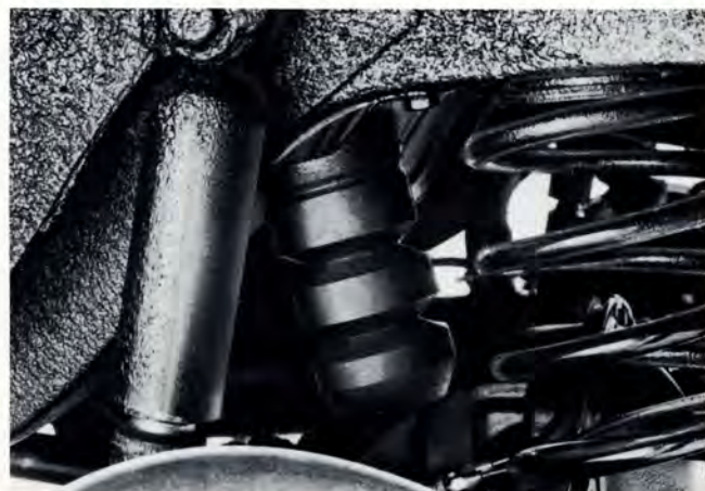
Auxiliary hollow rubber springs on the 145 supplement the rear coil springs to limit vertical axle travel on rough roads.
