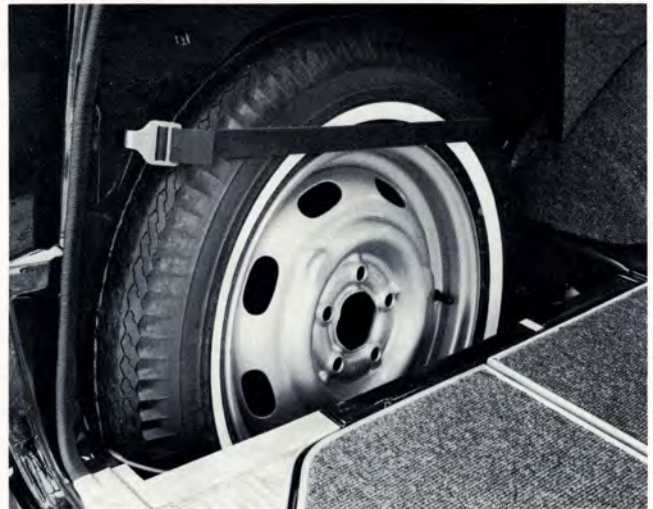
Vertical mounting of the spare wheel and tire in the left corner means the wagon doesn't have to be unpacked to change a flat tire.
