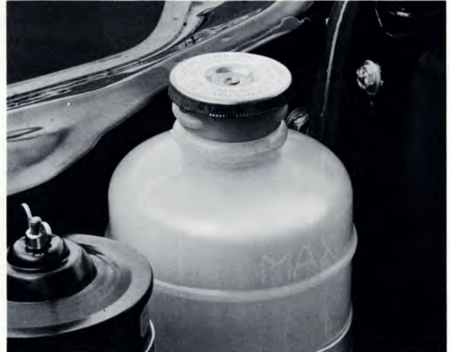
The sealed cooling system with 10 p.s.i. pressure has a transparent expansion tank for visual inspection of the coolant level.
