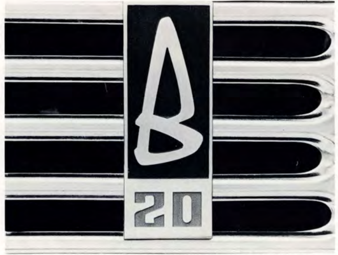
140 Series cars have a B-20 grille insignia, Volvo's designation for the 2-litre four-cylinder engine.
