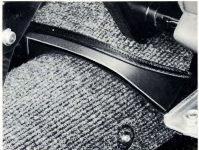
Rear seat passengers are kept warm with temperature controlled heat via extra ducts atop the transmission tunnel.
