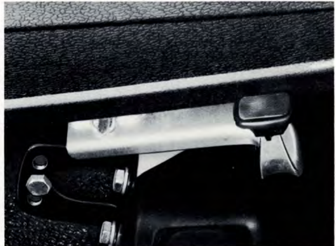
140 Series seats and the 164 passenger seat can be raised or lowered with this side adjuster. There is another adjuster in the front center of these seats and a position for moving the entire seat one-inch rearward.
