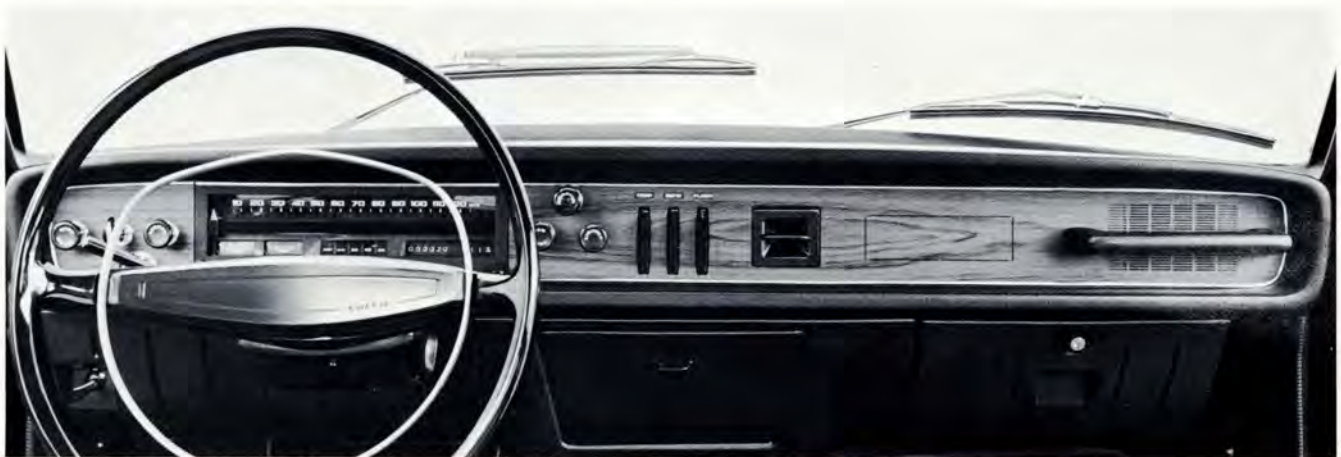
Glare free Volvo 164 fully padded dashboard has control knobs on the left and right of the instrument panel. Central heater controls are illuminated dials.
