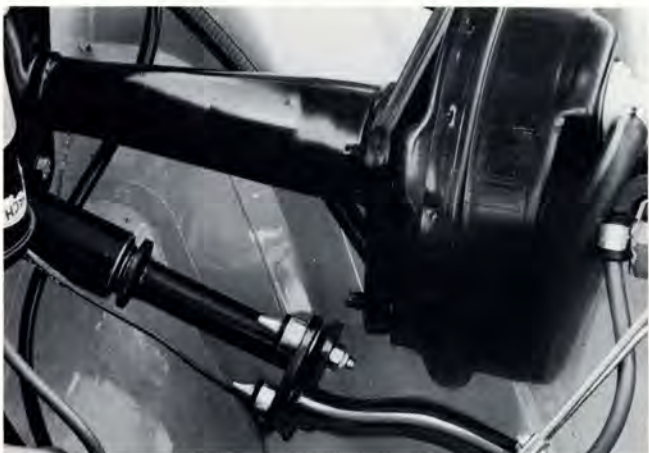
The 140 Series steering column is coupled together by steel pins suspended in hard rubber bushings to absorb shock.
