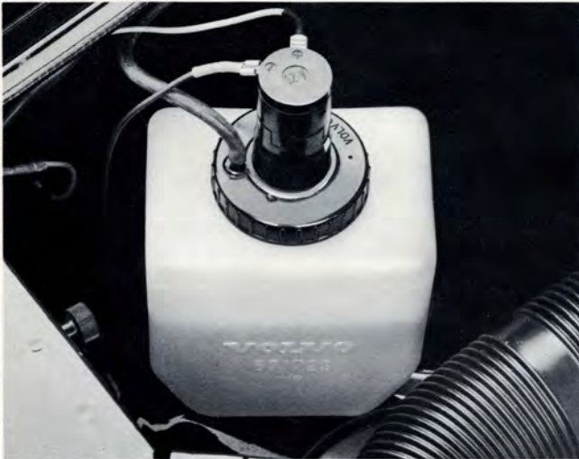
Powerful motor pumps cleaning fluid onto the windshield from a 1 1/2-quart container installed under the hood.
