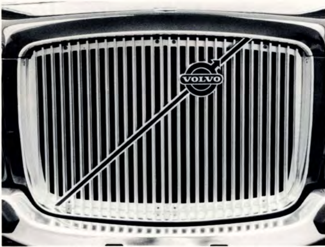
Distinctive 164 front end features a cast aluminum grille. The distinctive diagonal slash was adapted from classic six-cylinder Volvos of the '30s.
