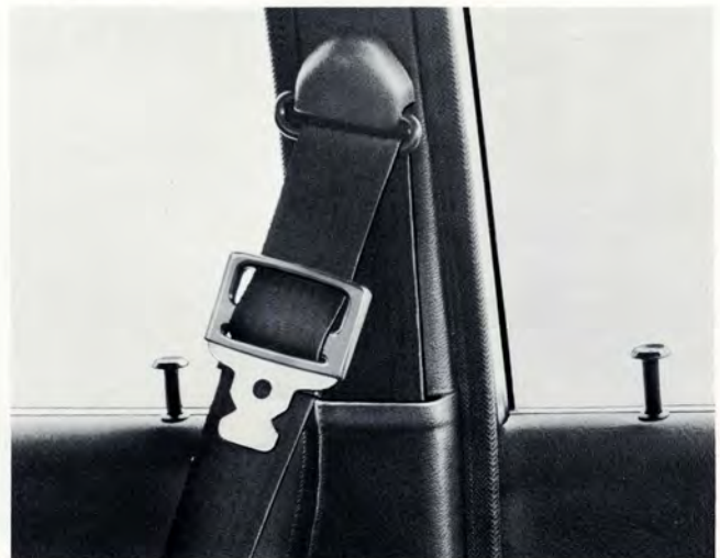
The inertia reel mechanism is fully enclosed in the center B-post. Occupants need only to pull out as much belt as is needed.
