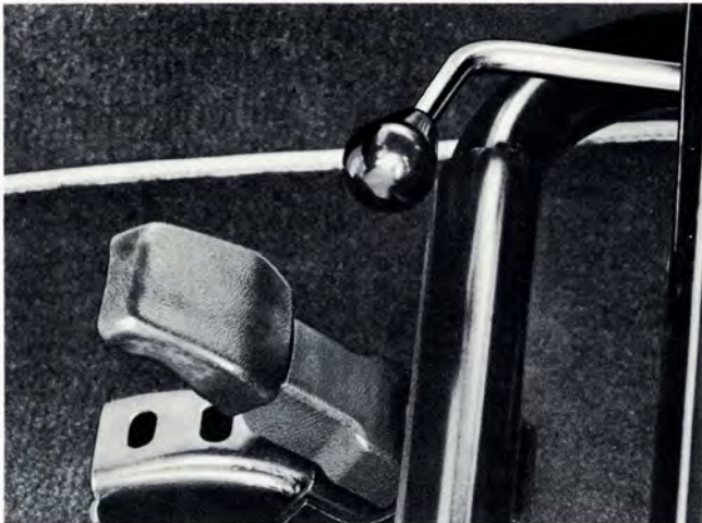
These two levers adjust the 164 driver's seat. The top lever is a back and forth adjuster only. The other, in the front center of the cushion, is used for moving the seat up and forward or back and down.
