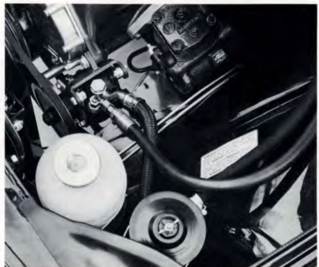
Power steering is standard on the 164. Hydraulic pump, top right, is belt driven. Fluid reservoir is at the bottom center.
