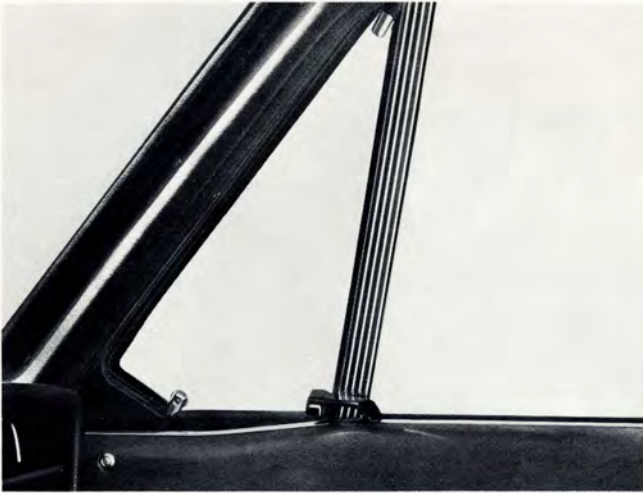
Redesigned door panels now enable the vent windows to be almost fully swiveled.
