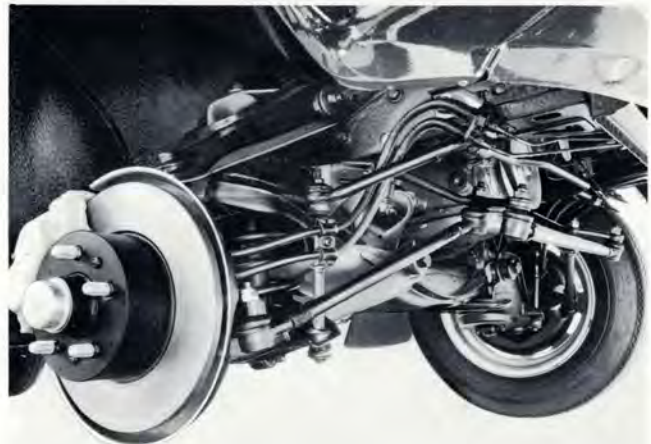
The 140 Series and 164 front suspensions are identical except for thicker springs and stronger shock absorbers and stabilizer bar on the six-cylinder car.
