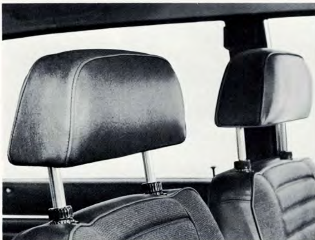
Head restraints on the front seats are raised 2\frac{1}{4} inches on 1970 models. They can be further raised to suit any occupant's height or removed to convert the Volvo seats into twin beds.
