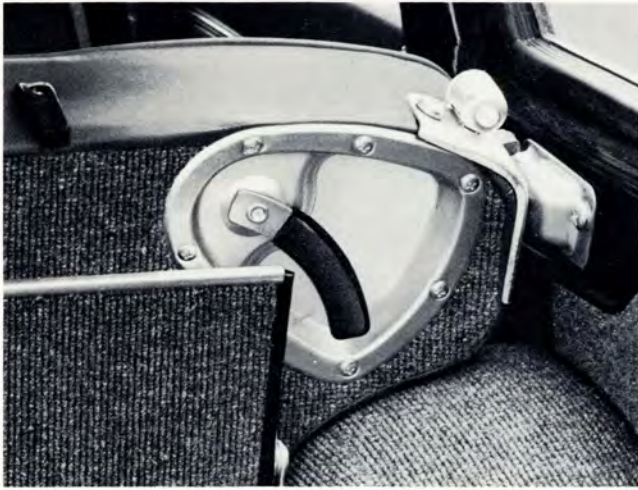
Back of the full width rear seat is upholstered with durable carpeting material. The folding levers are recessed for safety to prevent accidental opening.
