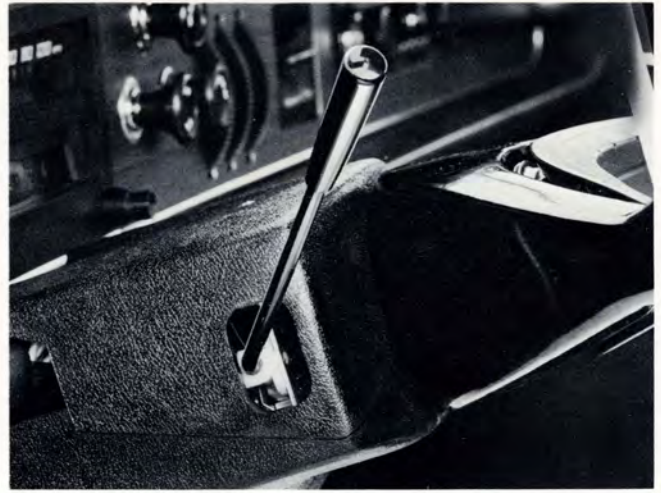
A lever mounted on the steering column gives mounted lever fingertip operation for dimming highbeams and operating directional signals.
