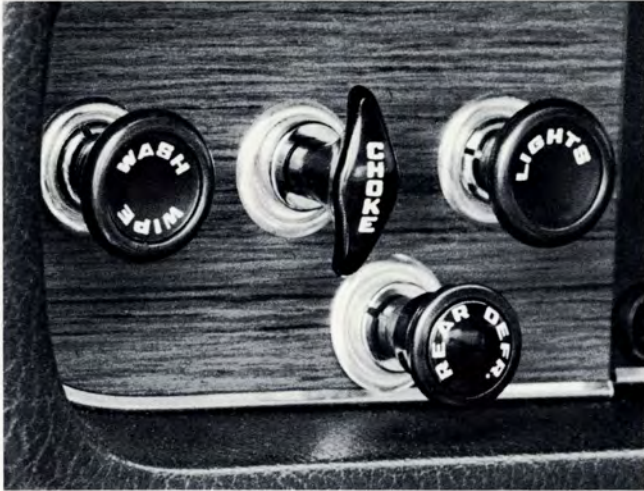
164 dash is finished with a wood grain pattern. The windshield washer has a spring loaded switch to prevent being left on accidentally.
