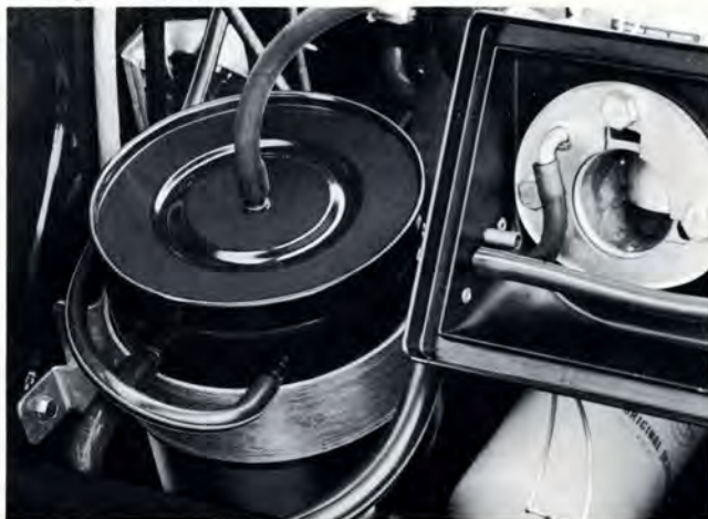
Part of the evaporation control system in this canister where gas fumes are mixed with filtered air before being sucked into the carburetors.
