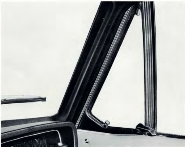
The interior windshield surround and corner posts now have a glare free cover.
