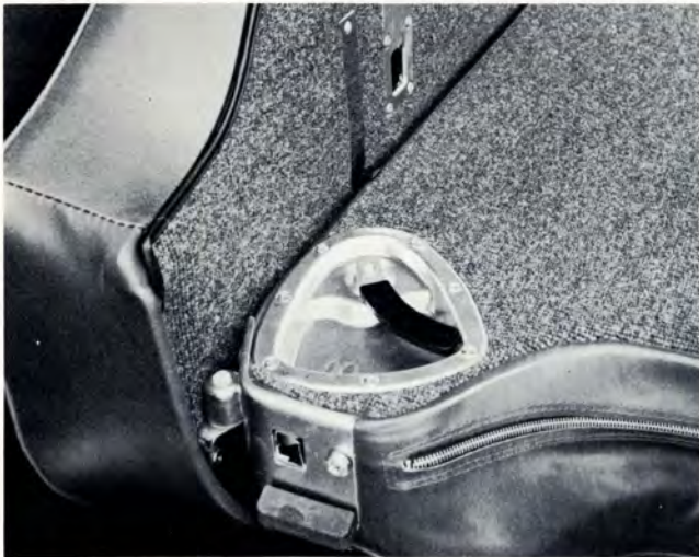
A handle on either side of the backrest turns to fold the seatback flush with the floor. Folding this seat does not limit front seat travel.
