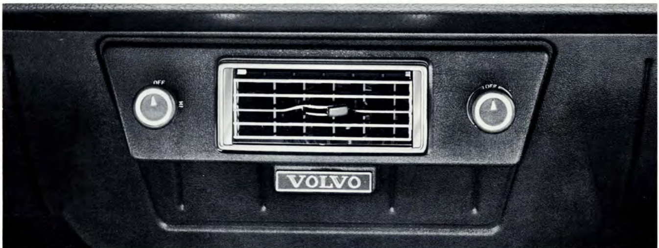
Custom air conditioning with redesigned ducting for increased cooling power is optional. Controls in this center panel adjust the temperature and blower speed. Additional
