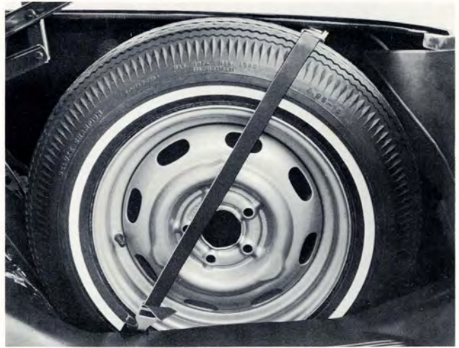
A recessed area enables vertical mounting of the spare tire for easy accessibility.
