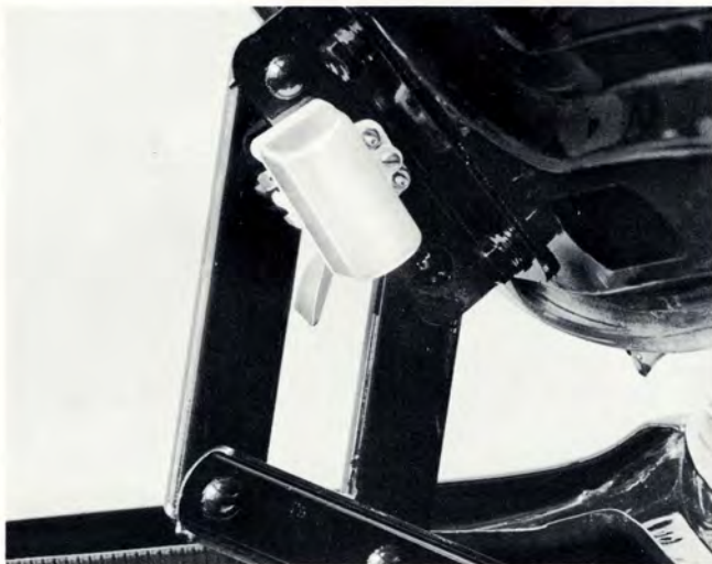
The 164 is equipped with an automatic light in both the trunk and engine compartments.
