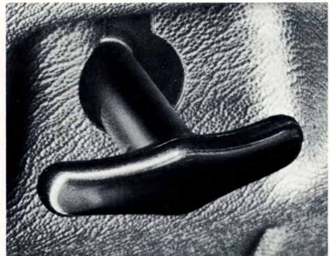
An inside hood release is supplemented by a safety latch under the hood.
