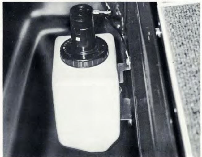
Reservoir for the electric rear window washer is stored in the side underfloor compartment. The container holds 1½ quarts of cleaning solution.
