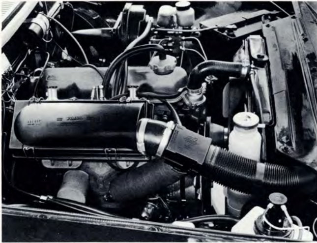
Two air intake branches, drawing hot air from around the exhaust pipe and cool air from the front of the car, meet at a coupling in front of the air cleaner housing.
