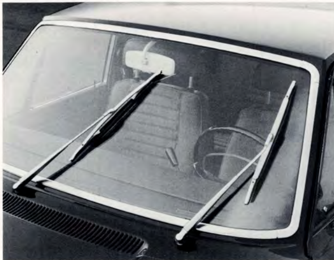
Volvo's 1250 square inch windshield is kept clean with full-sweep 16-inch wipers. Double laminated windshields on 1970 cars are bonded to the body.
