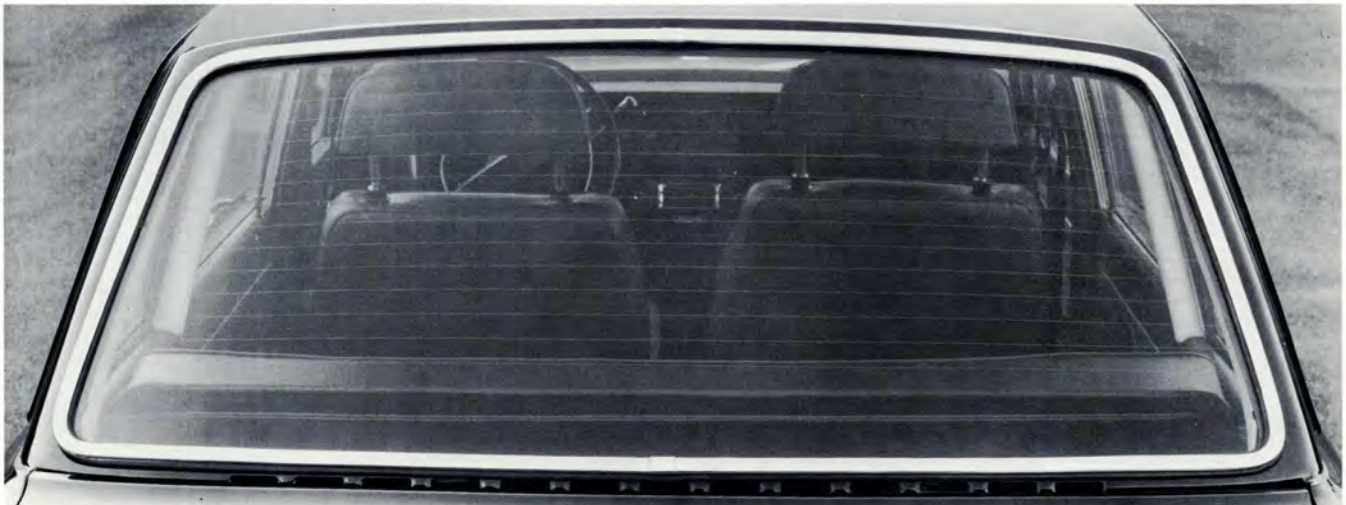
All Volvo models now have rear windows that are electrically defrosted. Special heat-conductor wires across the tinted glass are controlled by an illuminated dashboard
