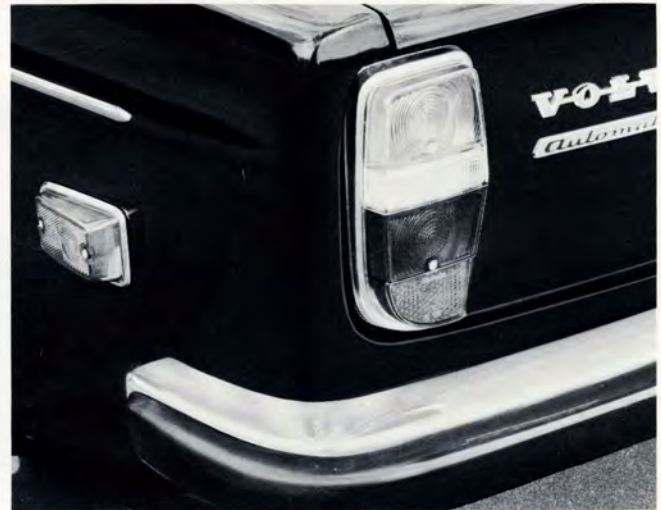
Rear lighting units are set at the extreme corners. Wrap-around bumpers front and rear are protected with hard rubber inserts.
