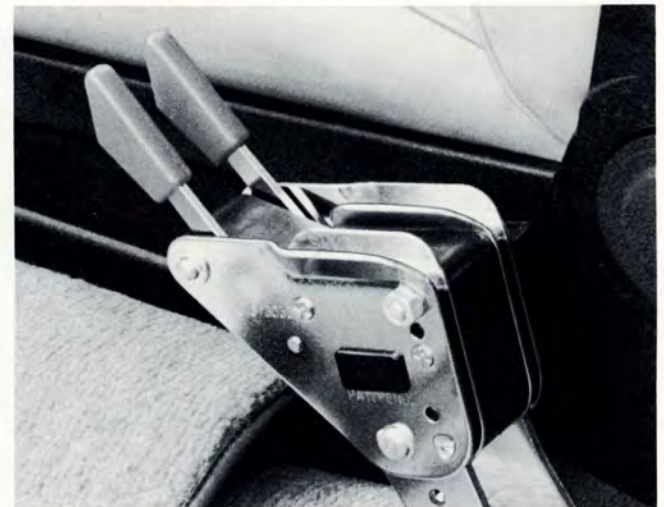
Driver and front passenger one-piece shoulder/lap belts lock into a quick release center mount with one-hand operation.
