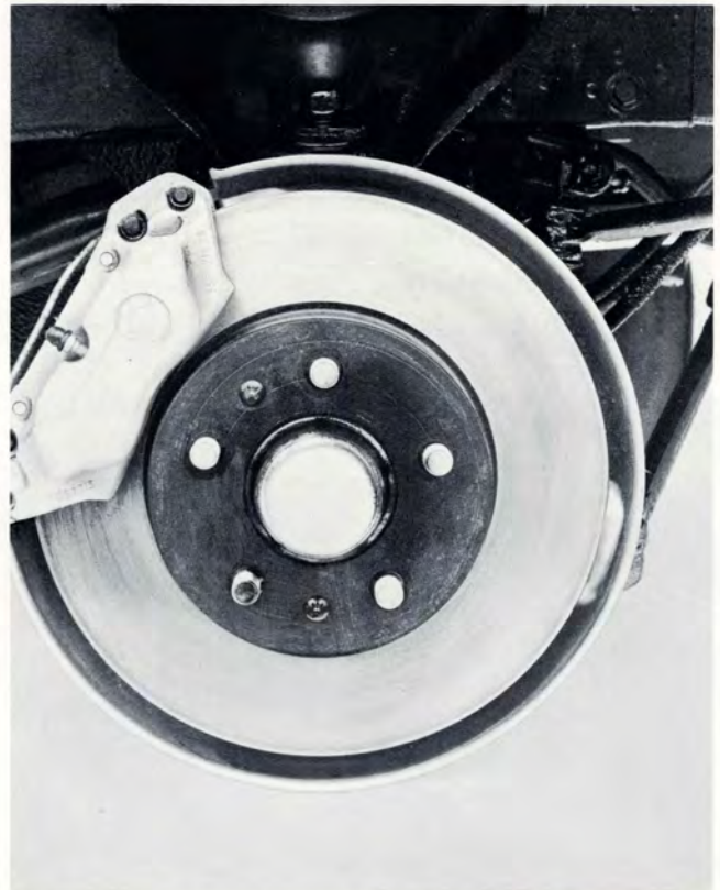
Front disc pads on the 164 are 35% larger than those on the 140 Series, compensating for the greater front end weight.
