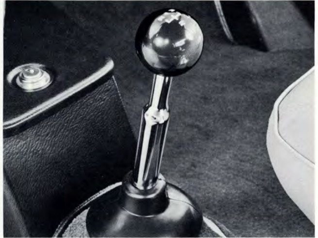
The 164 four-speed transmission now has a longer shift lever. It's set close to the driver's hand and requires only a short throw.
