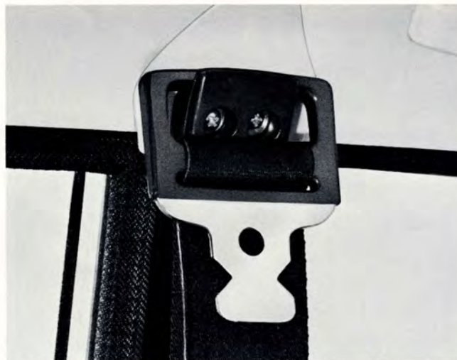
Volvo 3-point safety belts on 140 Series cars have a new, convenient-to-use combination hanger and adjusting handle.
