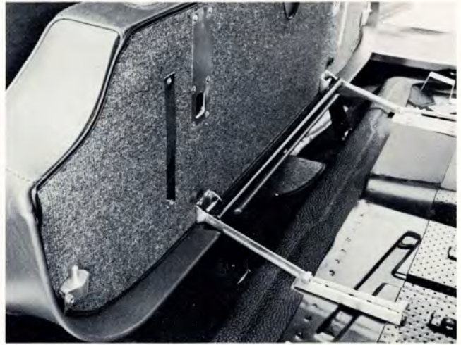
Pushing down on the front edge while pulling up from the rear unlocks the rear seat cushion so it can be raised and moved forward on rails.
