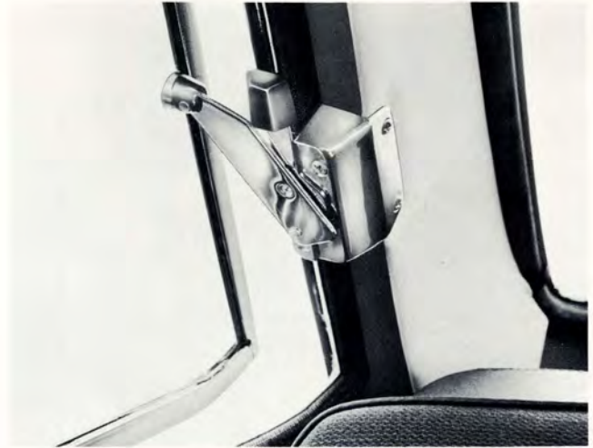
Hinged rear window of the 142 sedan can be opened for additional ventilation with a spring loaded latch.
