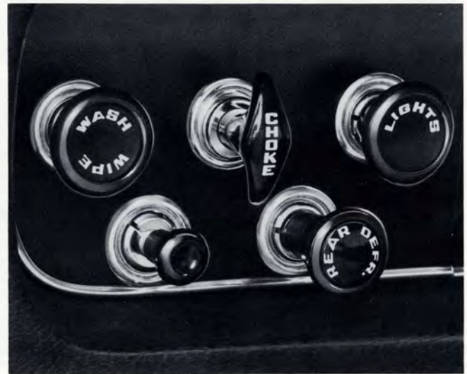
Knob on the lower left controls the 145 rear window wiper and washer. Alongside is the rear window defroster switch.
