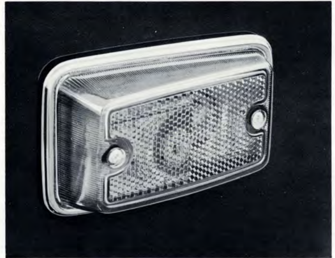
Side markers are illuminated on 1970 models. These lamps operate on the parking light circuit.
