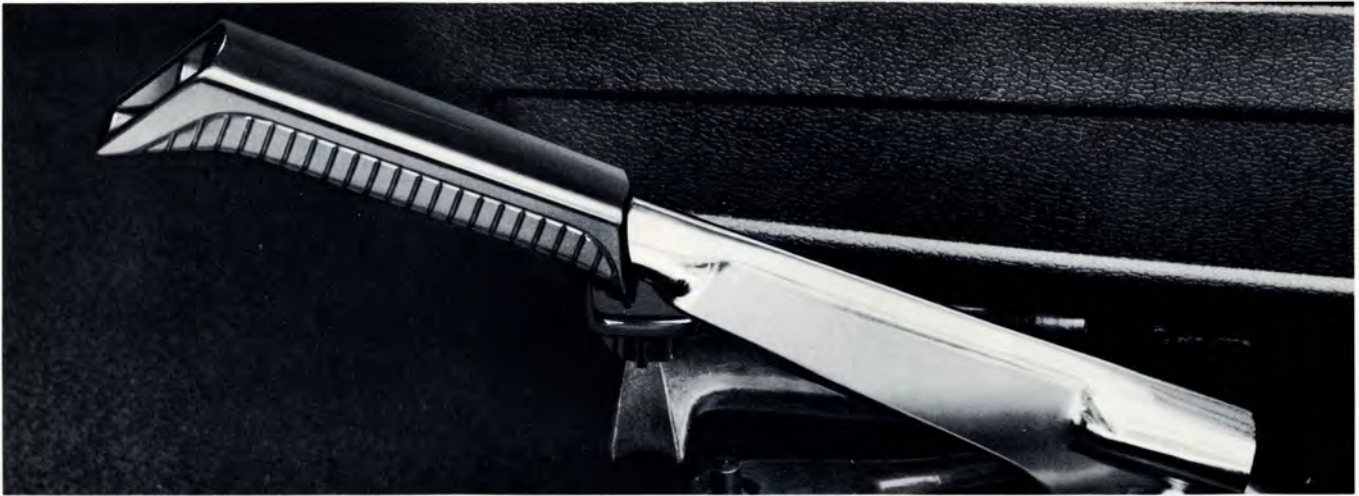
Hand brake lever sets between the driver's seat and door and has a dashboard warning light.
