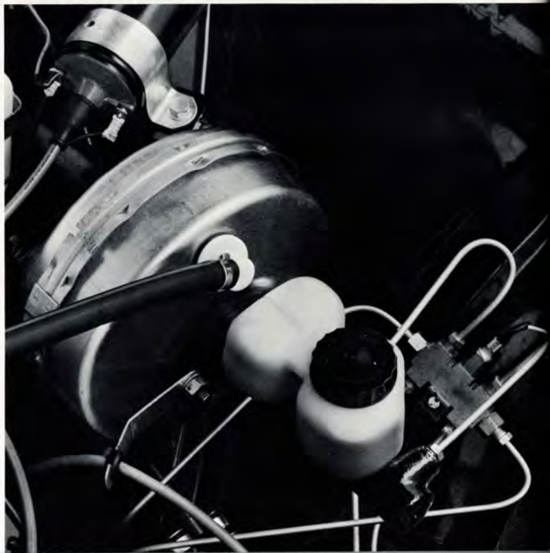
Hydraulic brake fluid level in the translucent twin reservoir can be inspected without removing the cap.
