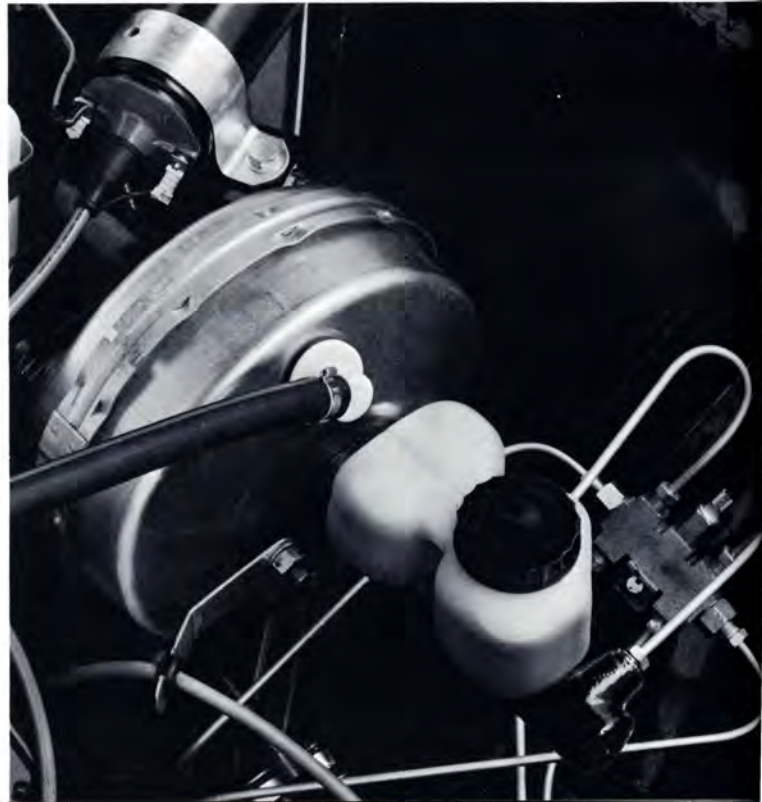
Hydraulic brake fluid level in the translucent twin reservoir can be inspected without removing the cap.
