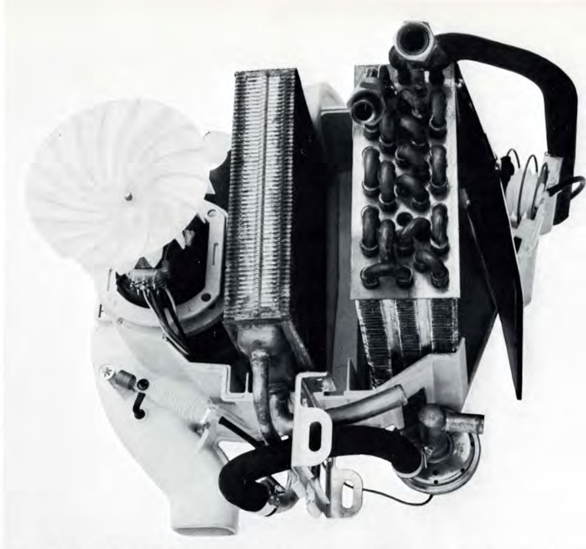
Exposed view of Volvo's new combined unit was taken from the side so only one of the two fans is shown. The heating core is in the center next to the evaporator unit for air conditioning. Because air passes through the evaporator before entering the heater core, moisture can be removed on damp winter days and the air then heated.
