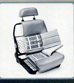
The seat frame is tubular steel. It supports a steel wire grid stretched between coil springs. The seat cushion is made of two layers of plastic foam with a stiffening layer in between. To give you support for your thighs on a long trip, the higher front edge of the cushion has softer foam. And the sides of the cushion and the backrest are raised for lateral support.
