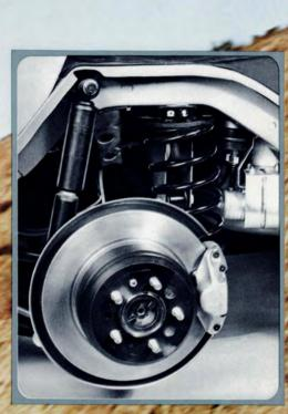
If the brakes on all four wheels of a car are connected to the same single hydraulic circuit, damage to the circuit could cause complete loss of brakes. To prevent that possibility, brake systems are divided into two independent circuits. If one fails, the other still works.
