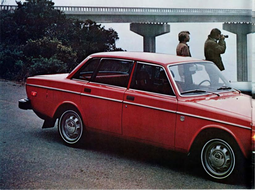
**SAFETY BODY** The fully-welded Volvo safety body combines six box profiles to form a protective cage around the passengers. Side struts running the length of the car and the large panel sec-tions are designed to provide lightweight torsional strength and to absorb energy in a collision.
