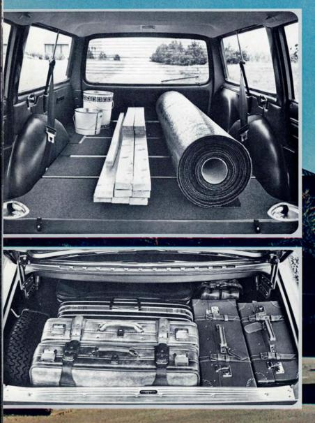
You're bound to notice it anyway, so here is a good place to point out a fault built into every Volvo. Perhaps it proves something about the company's philosophy of building cars. It's the high lip on the trunk. Makes it less convenient to load or unload heavy objects. Nevertheless, that piece of steel increases the structural strength of the Volvo body. It wasn't there in the first prototypes. Volvo engineers put it there, and have left it there ever since, because their tests told them to.
