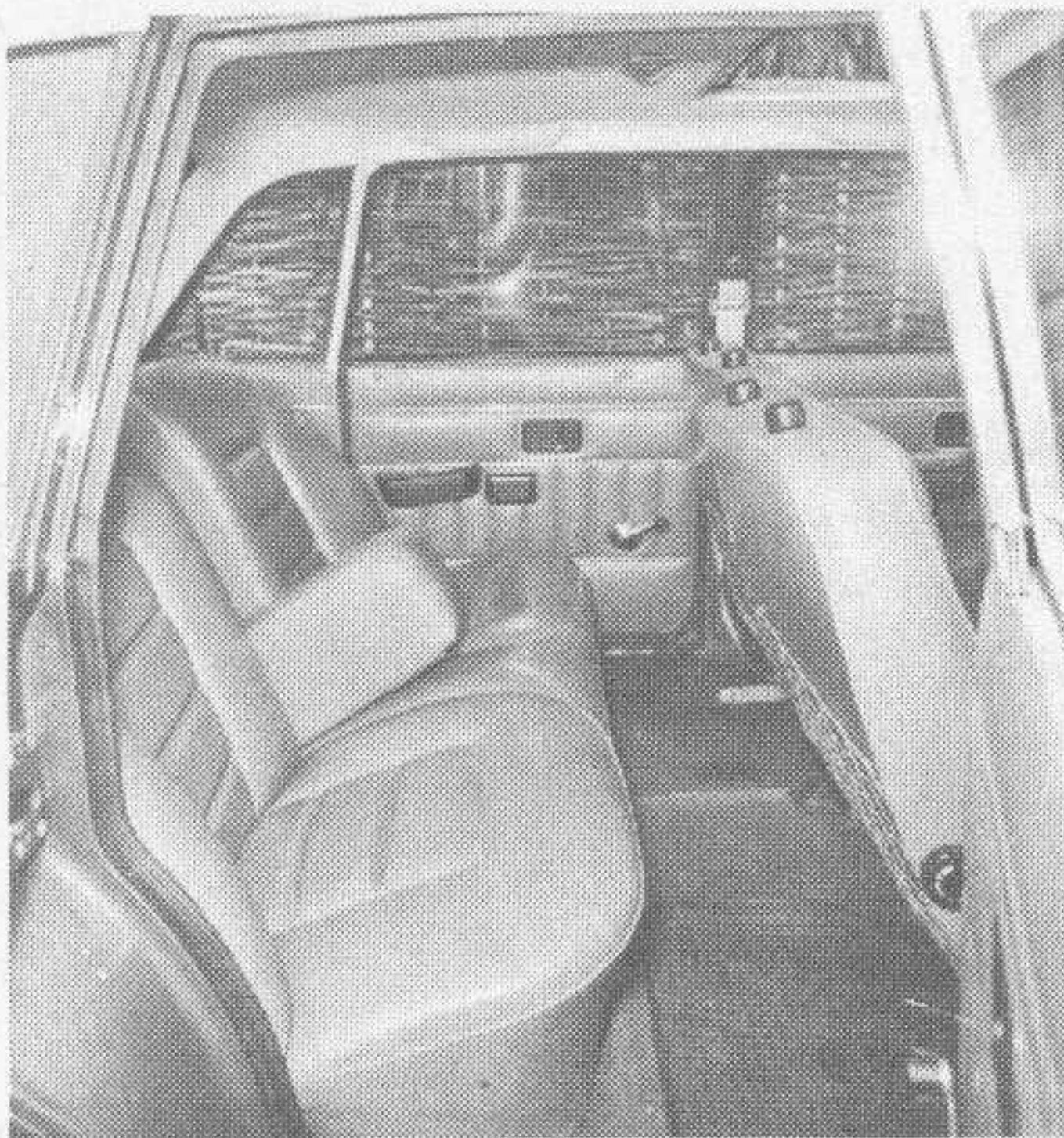
Above: In the rear compartment there is a large folding armrest in the centre of the shaped bench seat, and there are door armrests as well. String nets on the backs of the front seats provide further stowage for papers or maps. Below: A winding sunshine roof is fitted as standard on the 164E
