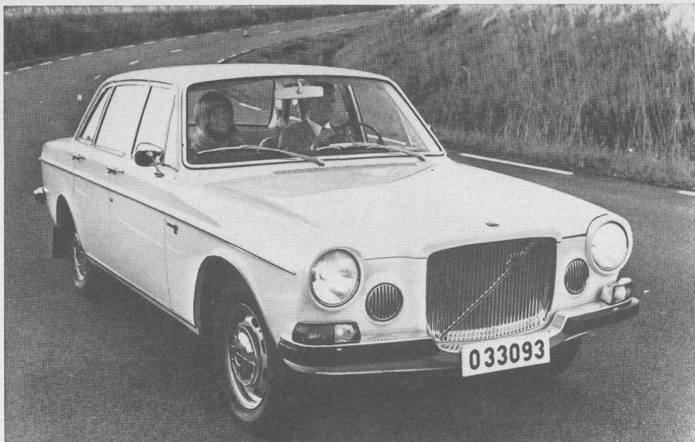
New 164 with 6-cyl, 3-liter engine has same body aft of windshield as 144 but longer front end and new frontal treatment.
