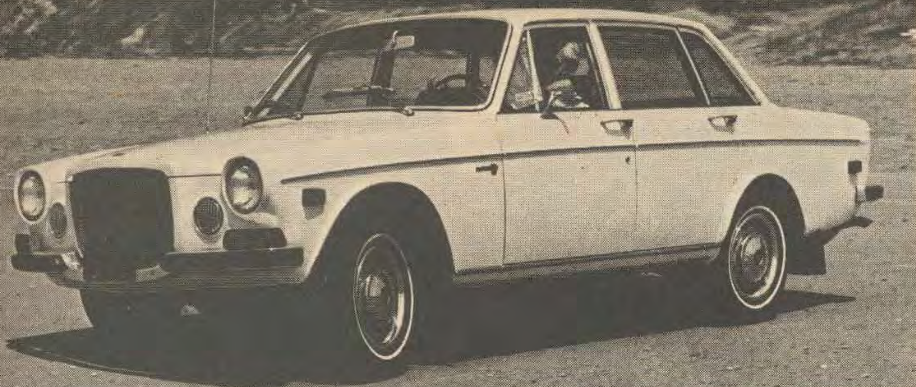
70-foot radius curve taken at 65-mph produces little lean. Note, though, the obvious understeer which is a desirable characteristic in a low-cube family sedan.
