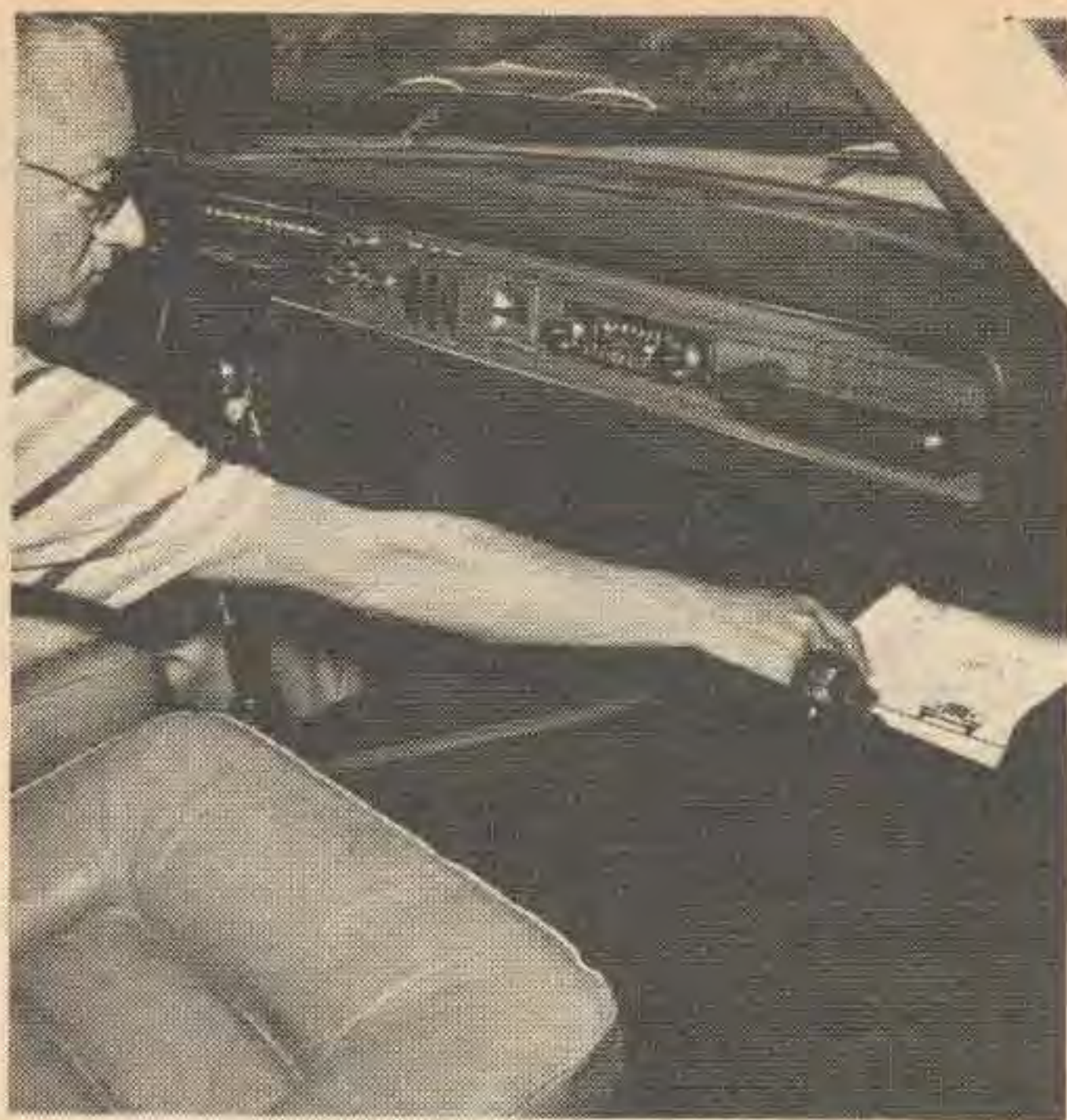
The glove box is a fair-sized reach for the driver but adjacent to it on the left is a handy panel that drops down to reveal every fuse in the car.
