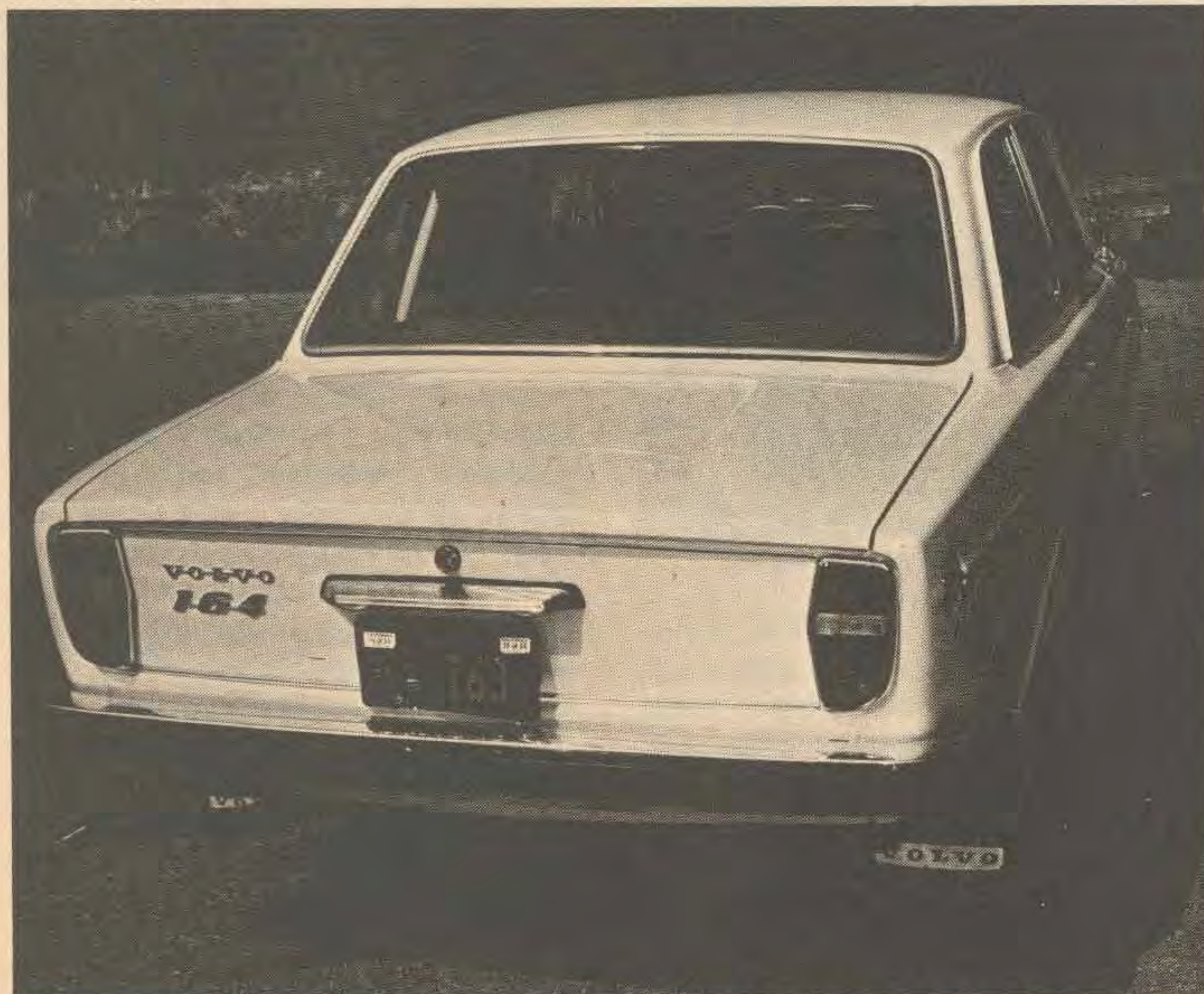
They are difficult to see, even from the driver's seat, but there are 13 wires imbedded in the rear window to demist or defog it. Trunk holds 23.6 cu. ft. of luggage.
