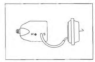
STEP NO. 25 — Locate the 3/8" vacuum hose routed from the vacuum pump thru the firewall into the passenger compartment. Cut this hose approximately 6 inches from the firewall. Slip clamps (12) over hoses and insert  $3/8 \times 3/8 \times 1/4$  vacuum tee. (21) Attach remaining vacuum tube, with clamp to tee, route to regulator and attach to "M" connector.
