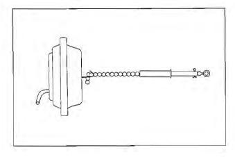
STEP NO. 13 — Slide metal bead chain guide outer tube as close to servo hook as possible and secure to chain with cotter pin. Crimp servo bead chain hook after installation.
