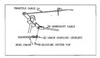
STEP NO. 11 — Install outer tube (13) of metal chain guide over bead chain. Do not as yet secure to chain with cotter pin.
