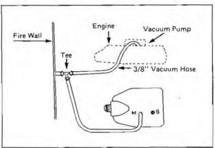
STEP NO. 26 — The vacuum tubing and wiring harness may be tied together or out of the way with plastic straps (16) to prevent damage from moving parts, hot manifold, etc. Also, excess wiring harness may be tied up under the dash area.
