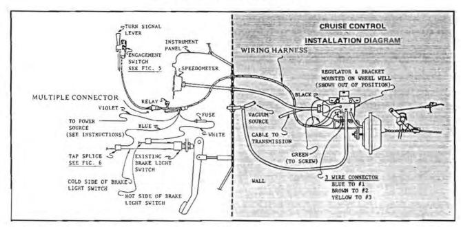
Referring to the installation diagram, note the location of each group of parts. The servo, regulator, and vacuum hose groups are located in the engine compartment. The engagement switch group is clamped on the turn signal lever. The wiring harness and cable group connect the various groups. Since the groups are connected with either cables, electrical leads, or vacuum hoses, it is suggested that the units be positioned in their approximate locations prior to actual mounting.
