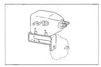
STEP NO. 15 — Attach both new cables to regulator and tighten nuts. Check both cables to see that:
