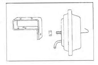
STEP NO. 9 — Position servo/regulator bracket mounting template (5) in place on right wheel well rib with tape and drill two (2) 11/64" holes. Remove template and attach servo and bracket with three 1/4 x 3/4 (19) washer head tapping screws with short leg of bracket pointing down. Tighten bracket screws securely.
