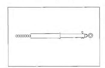
STEP NO. 12 — Attach bead chain to serve hook and adjust serve jam nut and nut/lock washer to remove slack from bead chain. Tighten jam nut and nut/lock washer assembly.
