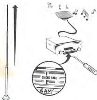
Pull out the antenna fully. Turn on the radio and check the function.
