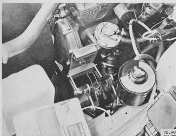
Remove the power pump pulley and the upper retaining bolt in the bracket. Push the pump downwards.
