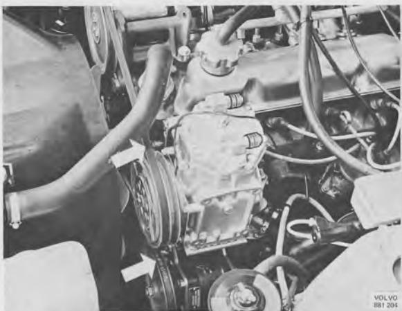
Install power pump, pulley and belt. Adjust the belt tension.
