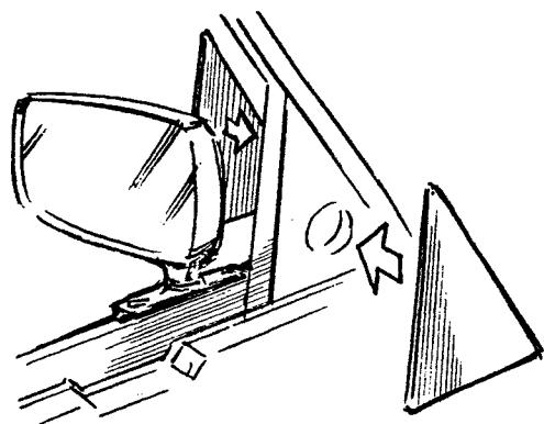
Re-fit the cover washers where the standard mirror was fitted.
