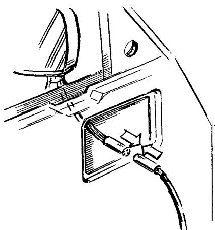
Join the end of the cable to the mirror cable connection.
