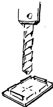
Drill a Ø 15 mm (19/32") hole in the centre of the cover washer.
