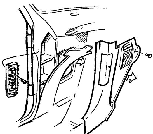
Remove the panel on the A-post and bend out the insulation board.
