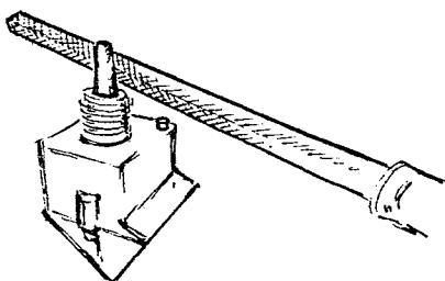
File off the lock stub on the control button.
