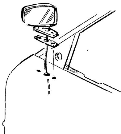
Place the rubber washer on the foot of the mirror and run the cable through the middle hole.
