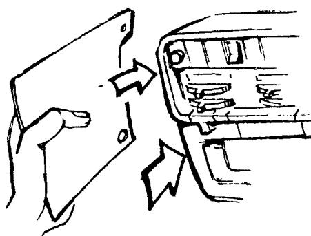
Push back the control panel into position and re-fit the panel against the heater.
