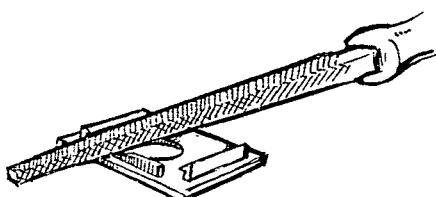
File the cover washer so that the button can be turned in different positions.
