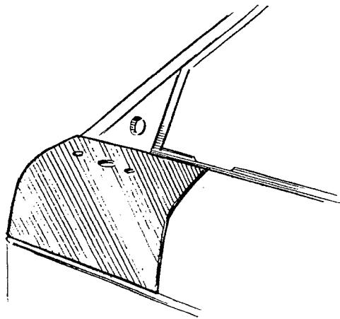
Place the template on the front edge of the door and mark where the holes are to be drilled.
