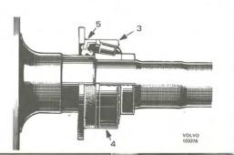
Install oil seal on shaft. (5)
