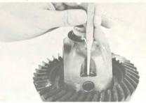
Remove shaft, gears, and washers. (19,15,16,17,18)
