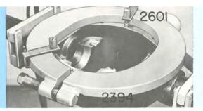
Install tool 2394 on casing.
