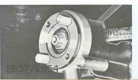
Install washer and nut on pinion. (24,25) Torque-200 to 220 foot-pounds.
