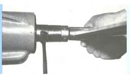
Check torque required to turn pinion. Torque- 4 to 10 inchpounds (old bearings) 9 to 20 inch-pounds (new bearings)
