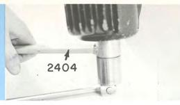
Install nut and washer on pinion. (24,25) Torque- 200 to 220 foot-pounds
