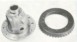
Install crown wheel on carrier. (21)
