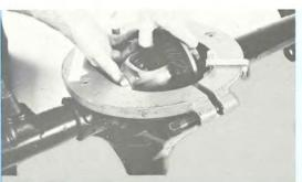
Lift out differential and crown wheel out. (12,21)
