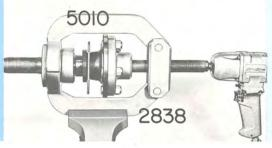
Press bearing and ring on shaft. (4,3)
