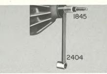
Install pinion with shims.
