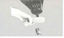
Remove pinion and front bearing.
