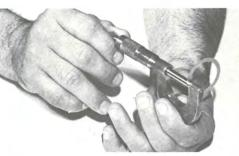
Measure shims to preload pinion bearing. Pre-load—0.07mm (0.003 inch)
