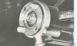
Remove nut and washer holding flange. (25,24,37/39)
