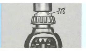
Install shims, bearings, and cups on carrier. (28,26,27)
