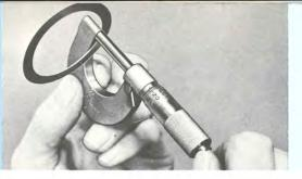
Measure shim to obtain shim equal to measurement.
