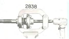
Pull bearing, ring, and oil seal off shaft. (4,3,5)
