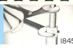
Install flange, washer and nut. (37/39,24,25) Torque- 200 to 220 foot-pounds.
