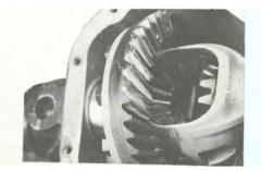
If axle is being repaired because of noise, check tooth pattern.
