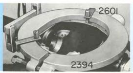
Install carrier in casing. (13)
