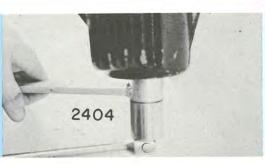
Install washer and nut. (24,25) Torque-200 to 220 foot-pounds.
