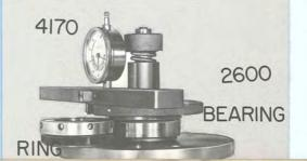
Measure adjusting ring and bearing.
