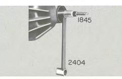
Install tools 2404 and 1845 on pinion. Pull pinion in.
