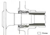
Remove inner seals for axle shafts.
