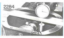
Adjust ring on pinion to dimension noted on top of pinion.
