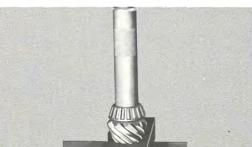
Install rear bearing on pinion. (29)
