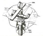
Place measuring tool 2393 in casing.
