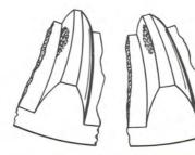
Incorrect pattern. Adjust backlash. If pattern is too far towards heel on driving side and too far towards toe on reverse side, pinion should be moved inwards.
