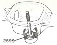
Remove front bearing. shims, oil deflector, and oil seal. (32,33,34,38/40,35)
