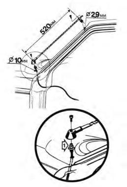
Measure up the upper hole, pierce and drill  $\Phi$  2.9 mm. Put a drop of rust protection oil in the hole. Screw on the antenna fastening and pull the antenna to the radio compartment.
