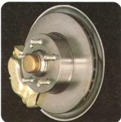
VENTILATED DISC BRAKES HAVE GREATER COOLING CAPACITY.
