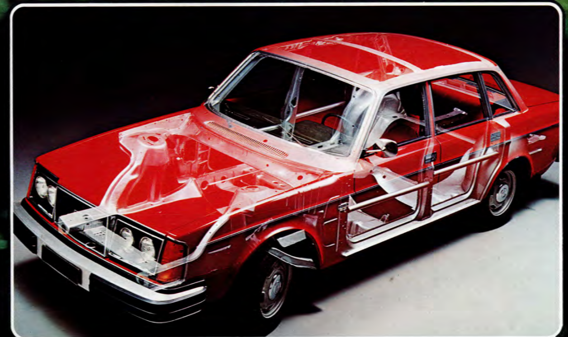
The basis for occupant safety is the unitized body with built-in passenger safety "cage." Each of its nearly 4,000 spot welds is strong enough to support the weight of the entire car.
