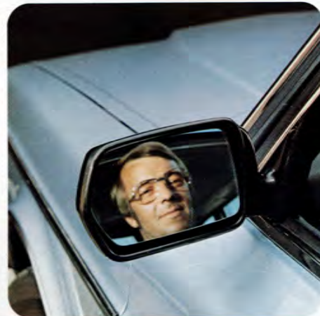
Power rear view mirrors make adjustments simple.
