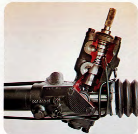
Power-assisted rack-and-pinion steering provides precise, positive control. It is standard on most Volvo models.
