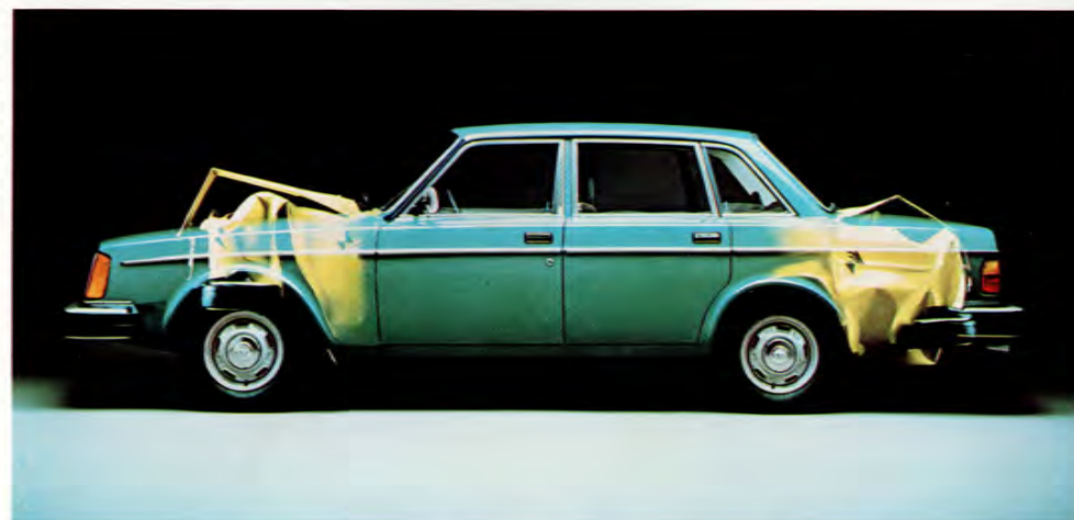
Crash-worthiness is the ability to absorb damage without harm to the passengers. To that end, both the front and rear of the all-steel Volvo unitized body incorporate zones designed to absorb and cushion impact energy instead of
