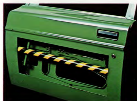
Obviously, not all collisions are frontal, so door reinforcement helps you in the event of a side collision. Each door is reinforced with strong tubular members attached to the door frames by a patented Volvo process.
