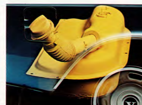
The fuel tank must be protected to prevent fire. In a Volvo, rear impact members create a safety zone around the fuel tank and combine with the energy-absorbing rear end to afford such protection. The tank is located well forward of the bumper, yet safely separated from the interior.
