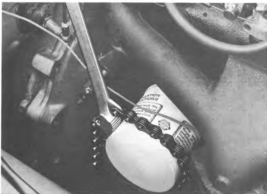
Demontering oljefilter B18, B20
