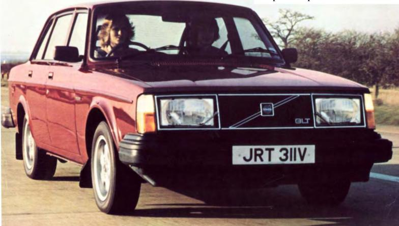
The 244GLT is also distinguished by the black front spoiler which adds to its stability and performance. Other standard features of the GLT include; power steering, ventilated disc brakes all round, sunroof, headlamp wipers/washers, tinted glass and all black interior.
