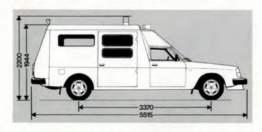
Dimensions Total length. 5515 mm and weights: Total width 1700 mm 1944 mm Total height. Wheel base 3370 mm Gross weight\_ 2220 kg
