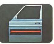
A steel tube is welded into every door to protect against sideswipes. Elimination of collapsible steering column teleof the vent windows has quietened the interior and strengthened the front doors.
