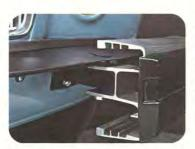
New, deeper bumpers are attached to hydraulic shock absorbers. They can take a bump at 5 mph.
