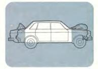
Front and rear ends are designed to serve as barriers in case you run into something or something runs into you. They both crumple at pre-determined rates to soak up the impact that would otherwise be passed on the passenger compartment.
