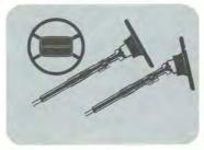
In case of front-end impact, a section scopes on itself. Pressure against the steering wheel moves it into a vertical position against which the driver's weight is more evenly distributed.
