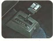
A trigger on top of the selector lever for the three-speed automatic transmission is designed to prevent you from shifting into "R" from "D" at 60 mph. And engaging a substantial repair bill.
