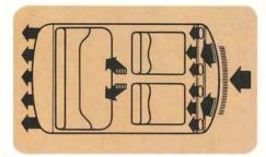
The powerful three-speed, ten-outlet heating/ventilation system. When we tested a Volvo travelling 35 mph, it maintained a constant  $+77^{\circ}$  inside when outside temperature was  $-13^{\circ}$ . In summer, it turns into a powerful ten-duct air conditioning system. It has cooled a 125° interior to 72° in 15 minutes with the outside temperature at 90°. The electric rear window defroster/defogger is powerful enough to melt a sheet of ice.
