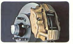
There's a power-assisted disc brake for each wheel. Discs resist "fade" due to heat build-up better than drum brakes. Front discs are specially ventilated to dissipate heat that can exceed 1100°F.
