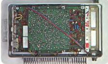
This solid-state computer monitors the fuel injection system and determines the precise fuel/air mixture required for every driving situation. Its decision is based on coolant temperature, engine rpm's, air temperature, air pressure and throttle position. It produces more efficient engine operation and a reduction of toxic emissions compared to this same engine operating with carburetors.
