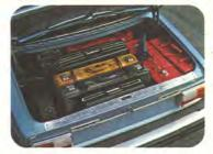
The trunk is box-like with 21.5 cu.ft. of useable space inside. You can pack your suitcases standing up and still get out the spare tire without unpacking.
