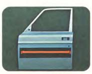
A steel tube is welded into every door to protect against sideswipes. Elimination of the collapsible steering column teleof the vent windows has quietened the interior and strengthened the front doors.
