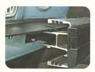
New, deeper bumpers are attached to hydraulic shock absorbers. They can take a bump at 5 mph.
