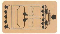
The powerful three-speed, ten-outlet heating/ventilation system. When we tested a Volvo travelling 35 mph, it maintained a constant  $+77^{\circ}$  inside when outside temperature was  $-13^{\circ}$ . In summer, it turns into a powerful ten-duct air conditioning system. It has cooled a 125° interior to 72° in 15 minutes with the outside temperature at 90°. The electric rear window defroster/defogger is powerful enough to melt a sheet of ice.
