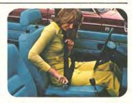
Self-adjusting three-point lap/shoulder seat belts are standard. They flex enough to permit normal movement but tighten
