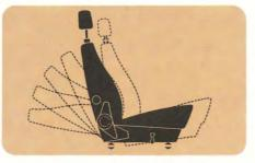
The bucket seat has a 7<sup>3</sup>/4" travel front-to-rear while the backrest reclines from vertical to nearly flat out. New locking devices make these adjustments permanent. Until a new passenger wants to re-adjust them.
