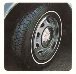
Steel-belted radial ply tires are standard. Tire industry tests show that radials perform better than conventional tires, and steel-belted radials perform better longer.
