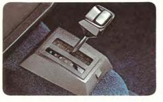
A trigger on top of the selector lever for the three-speed automatic transmission is designed to prevent you from shifting into "R" from "D" at 60 mph. And engaging a substantial repair bill.
