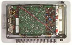
This solid-state computer monitors the fuel injection system and determines the precise fuel/air mixture required for every driving situation. Its decision is based on coolant temperature, engine rpm's, air temperature, air pressure and throttle position. It produces more efficient engine operation and a reduction of toxic emissions compared to this same engine operating with carburetors.
