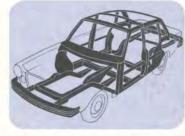
Six boxed steel pillars guard the 164 E. Steel supports stiffen the roof. Anti-intrusion bars reinforce the doors. Stronger bumpers protect the body.
