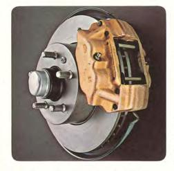
There's a power-assisted disc brake for each wheel. Discs resist "fade" due to heat build-up better than drum brakes. Front discs are specially ventilated to dissipate heat that can exceed 1100°F.
