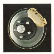
Warning light goes on if one circuit fails. Single circuit provides about 80 % of full four-wheel braking efficiency. Special rear wheel pressure relief valves prevent the rear wheels from locking before the front wheels during emergency braking.
