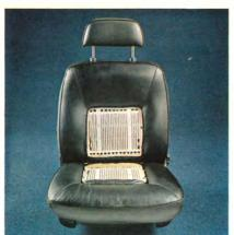
Inside the 142GL and the 144GL you sit on leather. The driver's seat is electrically-heated. Both front seats are fully adjustable up, down, back, forth, with reclining backrests. An adjustable lumbar support firms or softens the pressure against the small of your back. Passengers in the front can go up to 6'6". Above that, there's the sunroof.
