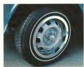
Wheels and tires Balanced, pressed steel wheels with safety rims. Chromed hub and lug nuts. 165SR15 steelbelted radial tires on 5Jx15" wheels.
