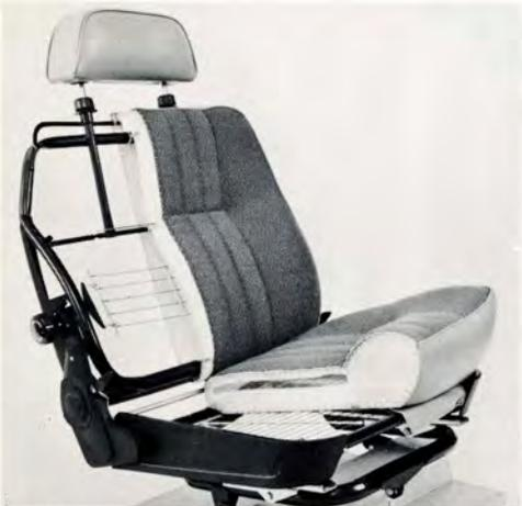
Further improved seats. The rubber straps in the seat bottom and lumbar support have been replaced by steel wires which are stronger and more durable. Helper springs have been added to the seat of all two door models so that the seatback automatically moves to the forward position when the catch is released.
