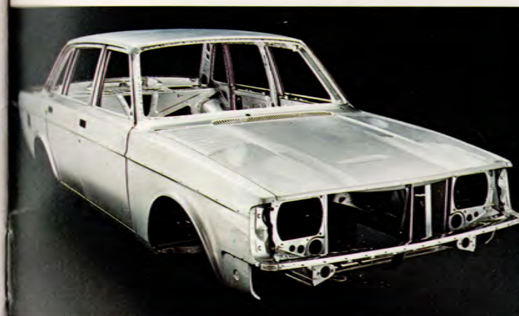
(Left) Fully-welded Volvo safety body combines box profiles to form a protective cage around the passengers.
