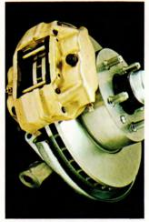
furnishes 30% of the car's total braking power while each rear wheel supplies 20%, you always have 80% of the car's braking power working for you even if one system fails.
