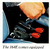
(from top to bottom) with: An electrically-heated rear window defroster. The control switch has 150W position so you can turn it up if a lot of snow is coming down. Steering shaft of the telescopic type. Not even marked deformation of the front end can be transmitted to the steering wheel. Three-point automatically retracting seat belts for the bucket seats. Three lap belts are provided for the back seat passengers.
