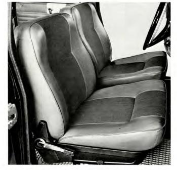
The front seats have firmer stuffing in the cushions and backrest. Reinforced, particularly durable upholstery. On the reverse side of the backrest there is a pocket for night duty coats. Tubular retainers under seats for batons.
