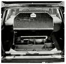
Under the floor of the luggage compartment there is an extra storage space with room for a fire extinguisher, warning flares, towline, rapid-action tyre chain links, warning flashers, safety triangles, car tools, spare fan belt and sand. Corresponding equipment is available in the four-door version. All the vehicles are fitted with a special jack which fits most makes of cars.
