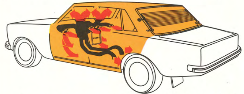
The heating/ventilation/air conditioning system has ten outlets: Two below the windshield; four adjustable nozzles on the dash; two outlets for the front floor; two for the rear floor.
