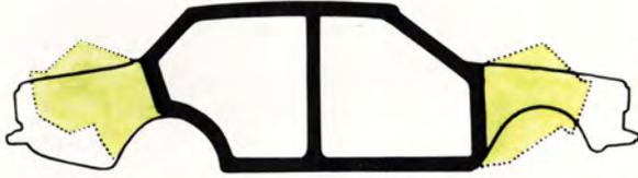
front and rear ends of the car. A substantial amount of the energy generated in a crash is absorbed before it reaches the occupant area.
