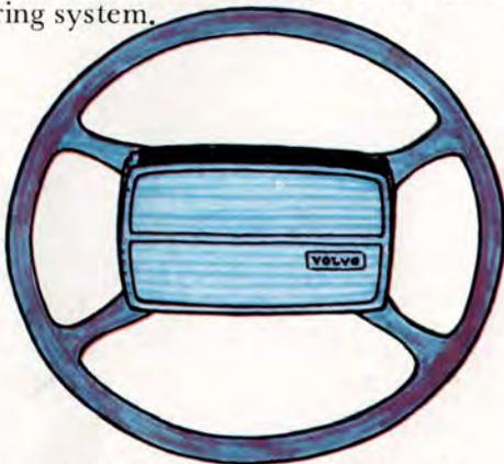
The steering wheel is connected to the steering column by means of a special "crumple-zone" unit. Under heavy pressure, this collapses and allows the steering wheel to align with the driver's body so as to spread
