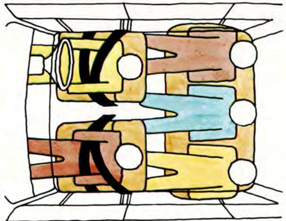
Today, all Volvo cars are equipped with three-point front seat safety belts. And the rear seats have safety belt anchorage points.
