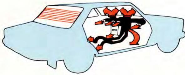
Volvo saloons have through-flow ventilation by means of air extractor vents at the rear. On our estate car, the extractor vent is located below the rear offside window. In both cases, the extractor vents have a check valve which allows air to pass through in one direction only. This means that exhaust gases can never penetrate.
