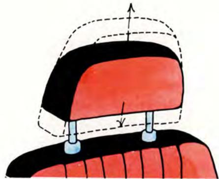
The adjustable head restraints safeguard the neck and spine from whiplash injuries should your Volvo be hit from behind. Height adjustment of the restraints is infinitely variable and quickly carried out.
