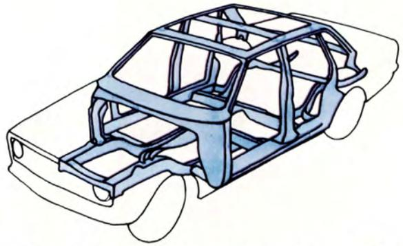
The body of a Volvo is designed so that the occupants are surrounded by a strong protective cage. And strong profile members enclose all body openings.
