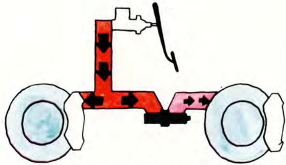
A relief valve in each of the brake circuits ensures the best division of braking power between the front and rear. This prevents the rear wheels from locking before the front wheels and therefore assists you in keeping the car under control even in emergency situations.
