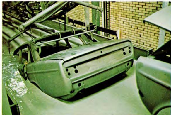
A Volvo is safeguarded by an unusually extensive amount of rust-proofing. For example, exposed parts of the body are protected by a layer of zinc (hot-dip galvanized).
