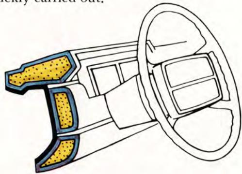
The entire occupant area is free from projecting controls and all hard surfaces are clad with safety padding.
