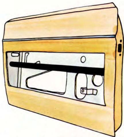
To give extra protection from side impact, the doors have a built-in anti-intrusion bar.
