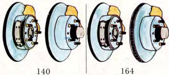
To reduce the risk of brake fade Volvo cars have disc brakes all round. Volvo uses disc brakes because they can be cooled more effectively. And on our most powerful cars (Volvo 164 with 145 or 175 h.p. SAE) Volvo uses a disc brake system in which the front wheel discs have special cooling channels. On all Volvo cars the disc brake system is power assisted.
