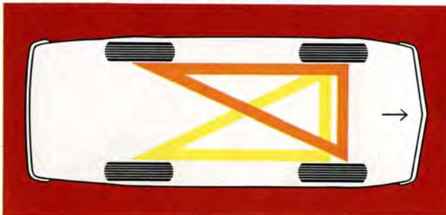
Each front wheel has a double set of brake cylinders and plungers, one set for each circuit. Therefore, each circuit brakes both of the front wheels and one of the rear. Which is why we call it a triangle-split system. You could lose 50 % of your braking system and still retain about 80 % of your braking power.
