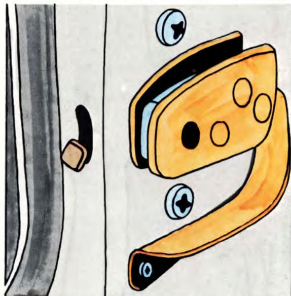
Volvo cars have door locks of burst-proof design which means that they stay closed even if the body is extensively deformed.
