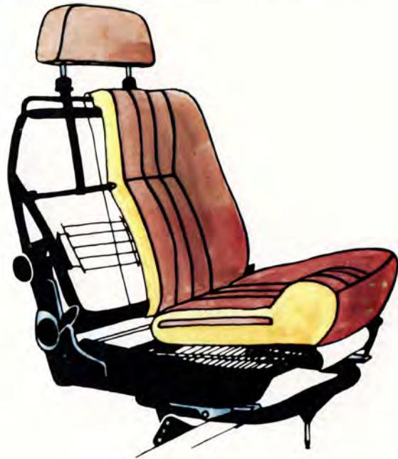
Correct support in the right places is achieved by using different densities of foam padding. The seat cushion for example supports the thighs, all the way out, and the front edge of the cushion is just right to give the correct support without applying undue pressure.
