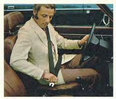
The Volvo self-adjusting shoulder/lap safety belt unwinds from an inertia reel when you put it on, and stores out of the way when you take it off.
