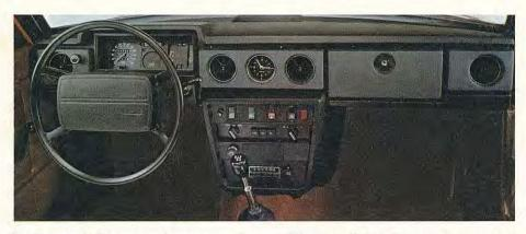
Instrumentation on the wagon is easily seen (white on black) and easily read (clocklike). Rocker switches are easy to work. At night the instruments light up with an intensity you control from a rheostat. You have no control over a warning light that lights up when low beams, brake lights, taillights don't.
