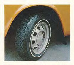
Tires on the wagon are white sidewall radial ply, just like the sedans. But to accommodate the heavier loads in the 145, Volvo fits a larger size 175 SR 15.
