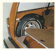
The spare tire tucks away in the side. If you have a flat and the wagon is loaded, you don't have to move the whole load to get at the spare. Underneath the cargo but not out in the open.
