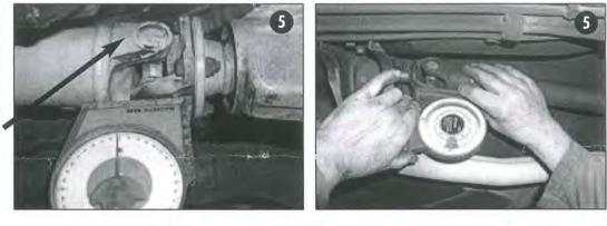
Once you have your measurements, remove one torque rod at a time and replace it with the new IPD adjustable torque rod. Do not remove both torque rods at the same time. To start, adjust your new IPD torque rods to the same length as the factory units and install them into the vehicle one at a time.
