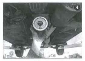
Measure the driveshaft angle at the carrier bearing and differential. Note that when measuring you should take care to have the angle finder flatly placed against the u-joint flange at the differential and carrier bearing, not places against the flange on the drive shaft.
